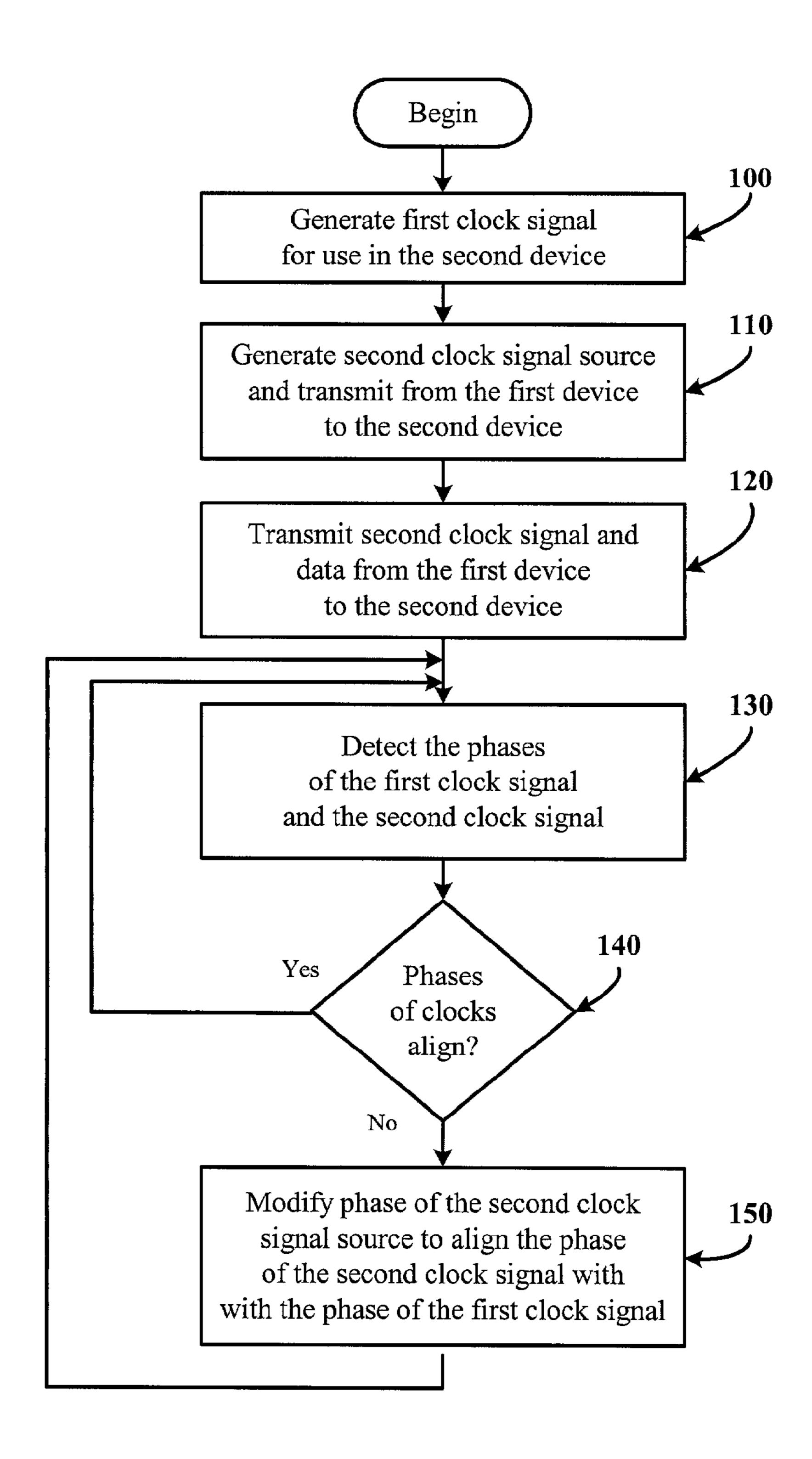
Figure 1 Phase Alignment Process
