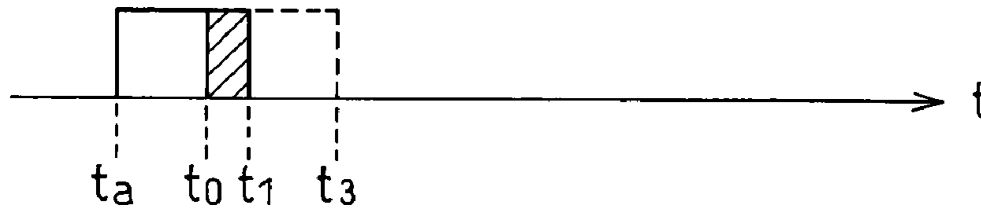
RETURN TIMING OF REFLECTED WAVE FROM SHORT-RANGE TARGET
