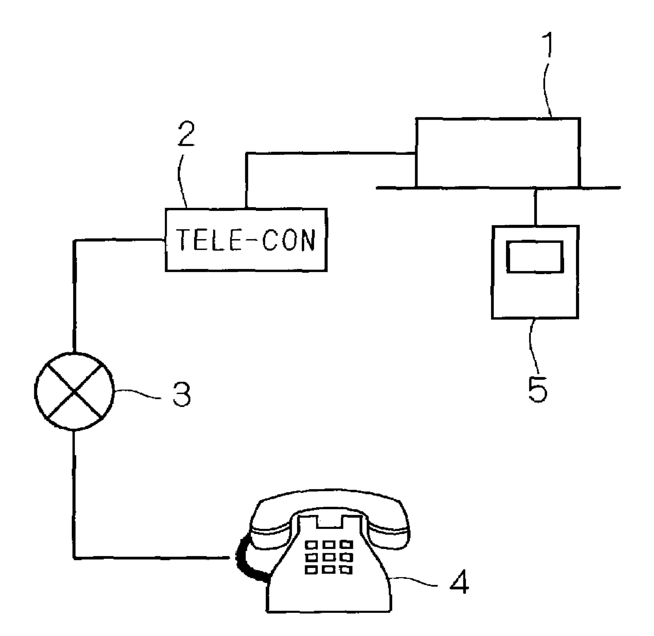
REMOTE OPERATION SYSTEM FOR AIR CONDITIONING APPARATUSES, REMOTE OPERATING METHOD FOR AIR CONDITIONING APPARATUSES AND BASE STATION FOR PERFORMING REMOTE OPERATION OF AIR CONDITIONING APPARATUSES
