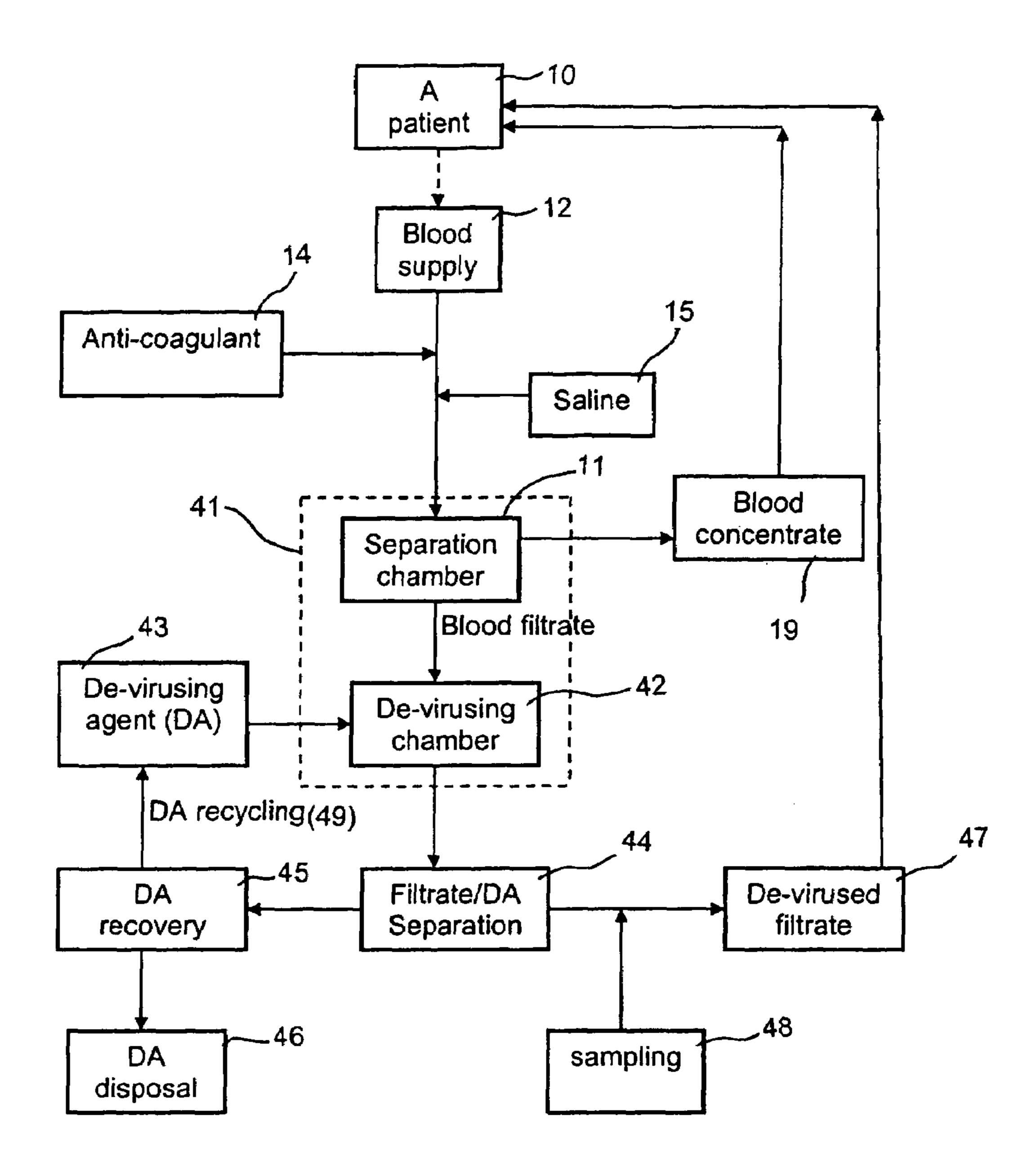
Within the broken lines (- - -) is a separation chamber arrangement
