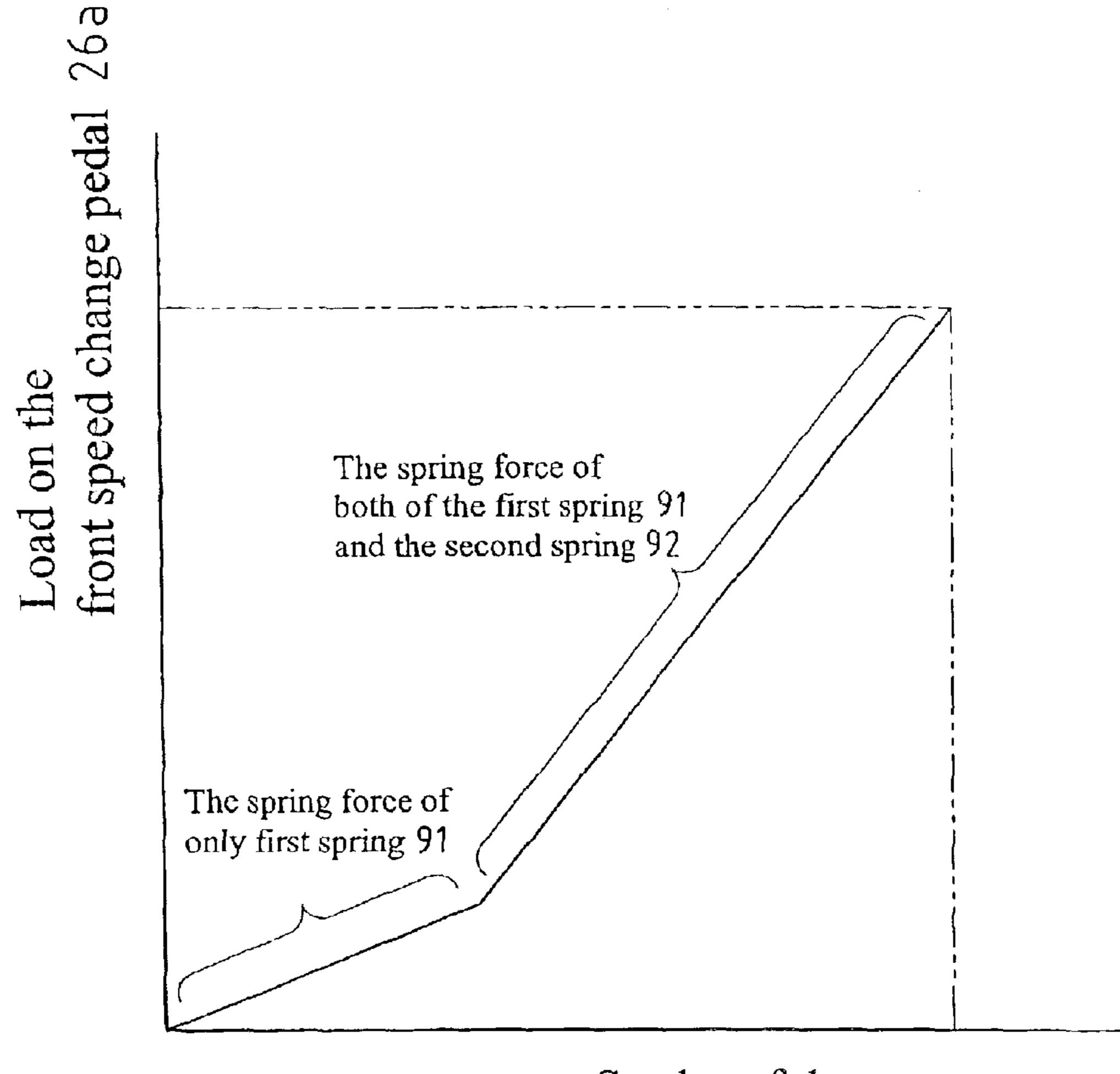
Stroke of the front speed change pedal 26a
