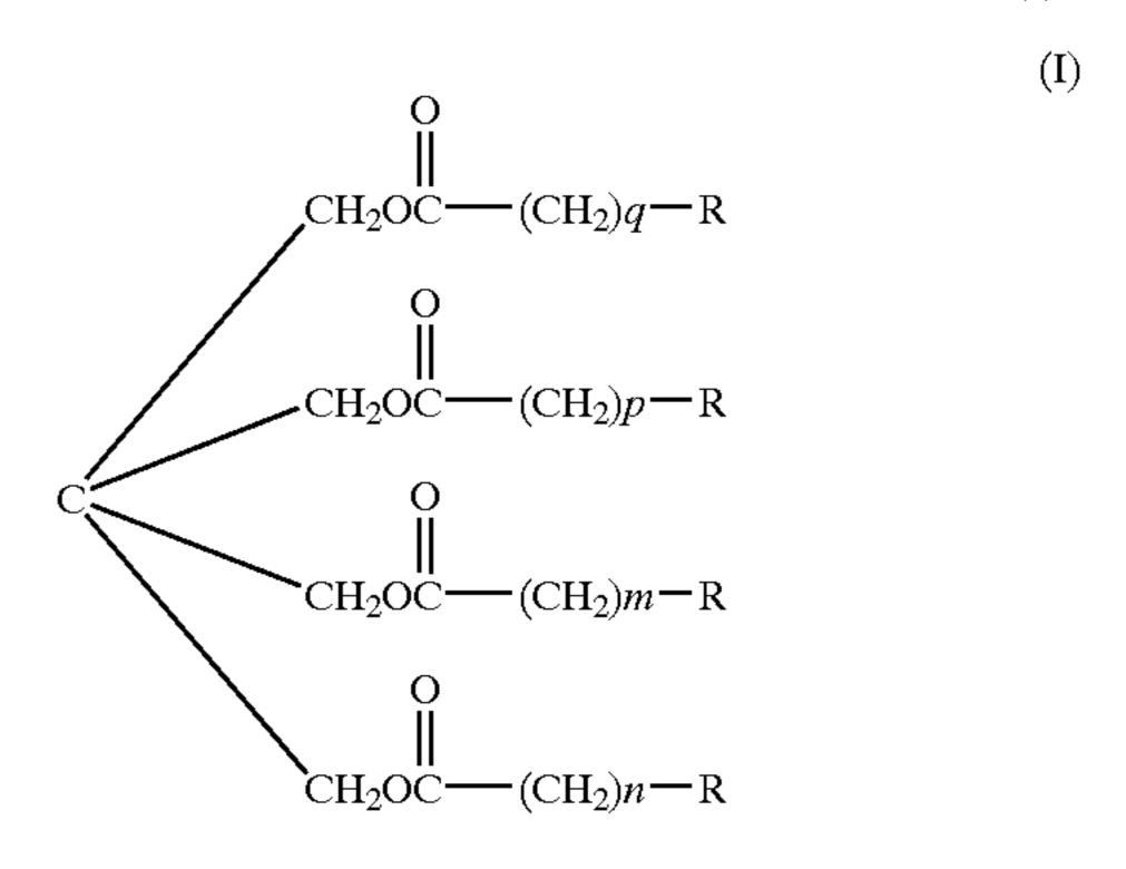
wherein p, q, m and n each represents a positive integer of 16 to 22 and R may be the same or different and each represents a hydrogen atom or a lower alkyl group having 1 to 4 carbon atoms. The electrophotographic toner is capable of remarkably enhancing the fixation strength of the toner and inhibiting the occurrence of voids during the printing and the occurrence of fuming and odor during the fixation.
