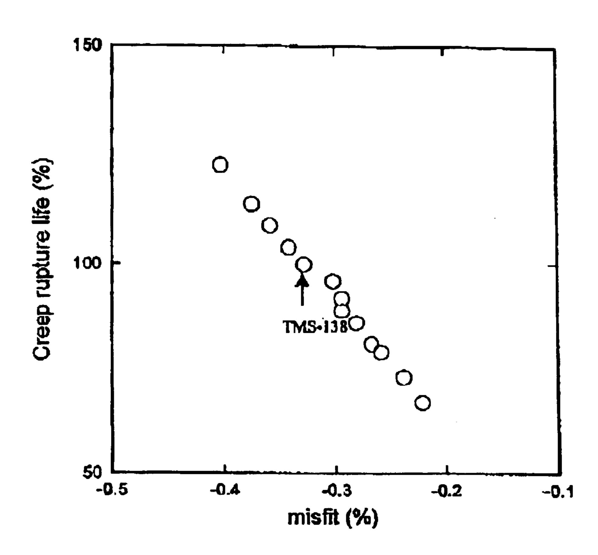
Relationship between change of the misfit in the alloy based on TMS-138 and creep rupture life of the alloy. (creep rupture life of TMS-138 is set up to 100%)
