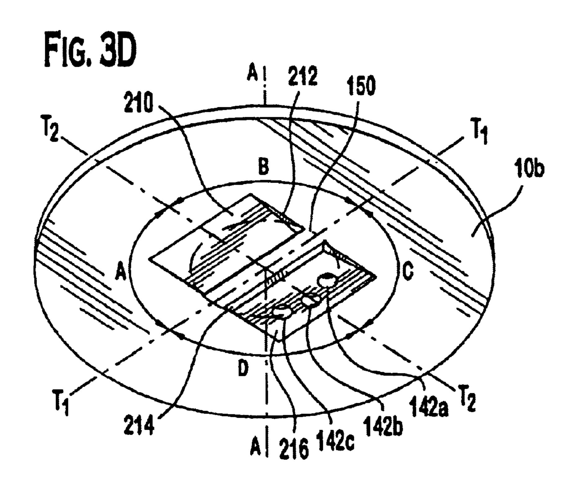
SPRAY PATTERN CONTROL WITH NON-ANGLED ORIFICES FORMED ON A GENERALLY PLANAR METERING DISC AND REORIENTED ON SUBSEQUENTLY DIMPLED FUEL INJECTION METERING DISC
