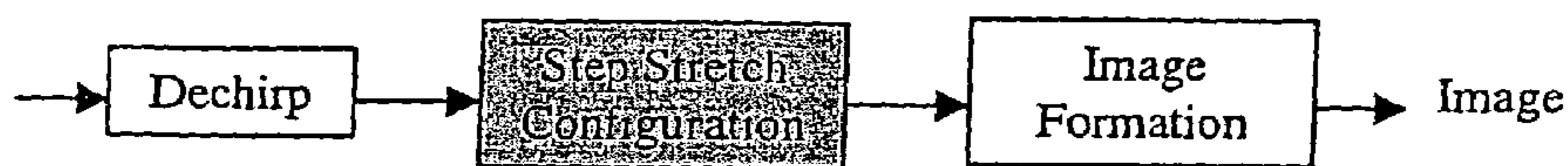
Fig. 4 Range sample combining block in the SAR signal processing chain
