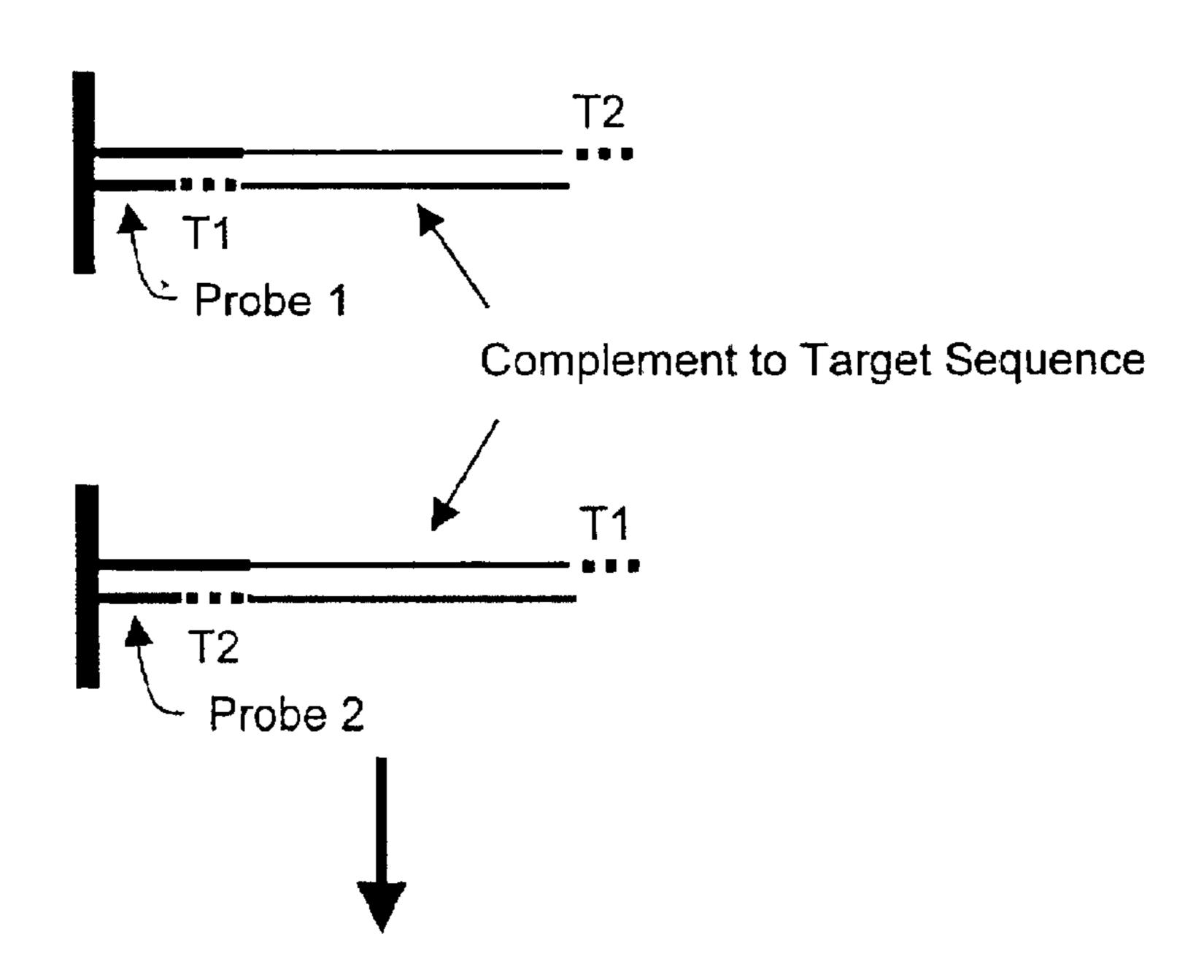
5) Ligate and wash with high stringency to leave one strand of target sequence on each of the two probes
