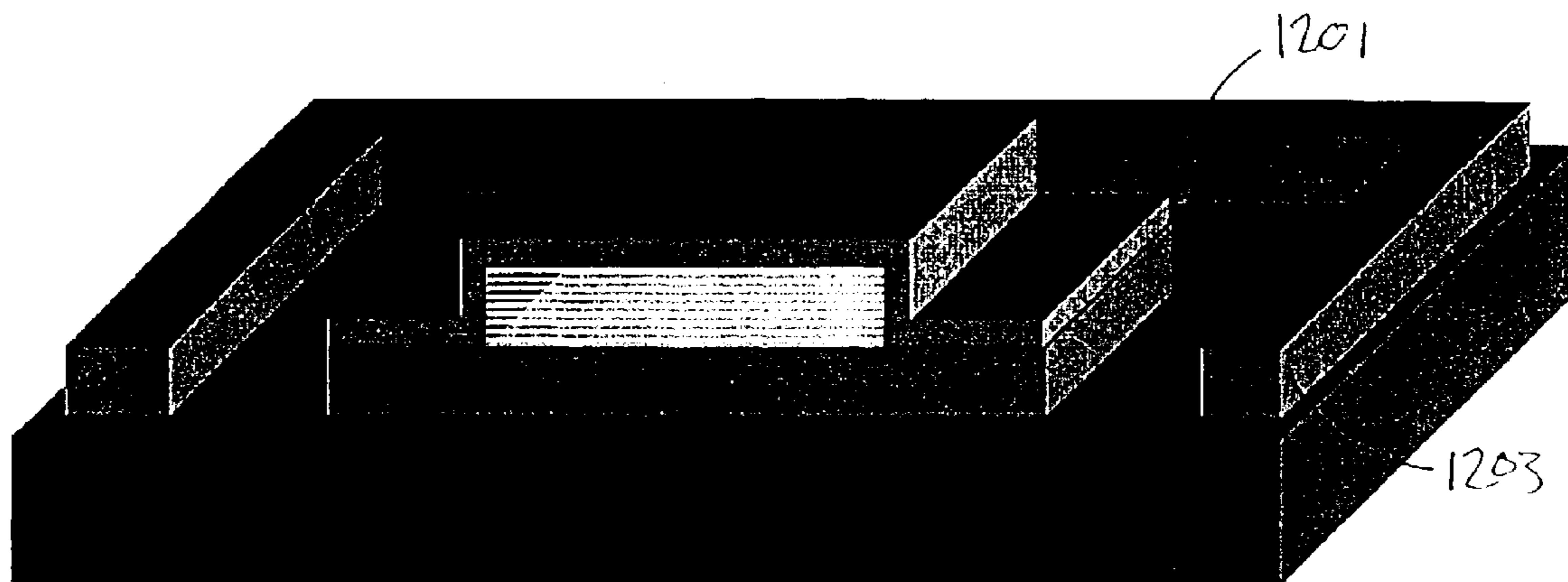
Via hole trench is etched through GaAs surrounding area of active circuitry.
