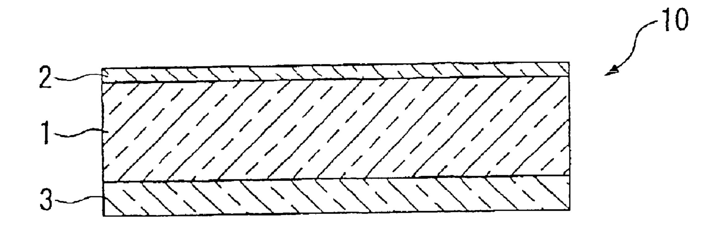
The present invention relates to an optical film having an antireflection property and having an optical correcting property such as a color tone correcting property or a near 5 infrared ray absorption property, and a process for producing
