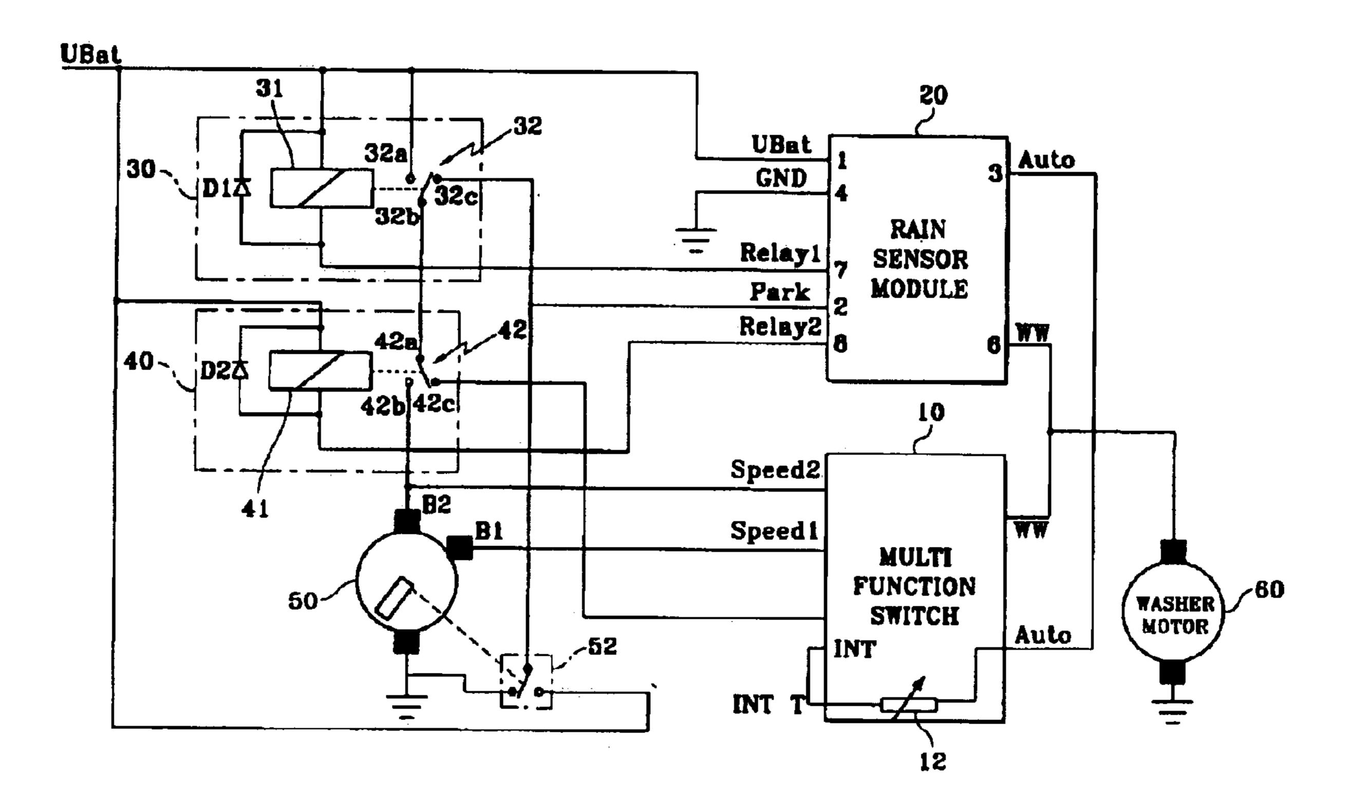
8 FUNCTION RAIN SENSOR KODULE 27 **P W B** Relay2 Speed2 Relayı Speed 1 GND Ŋ
