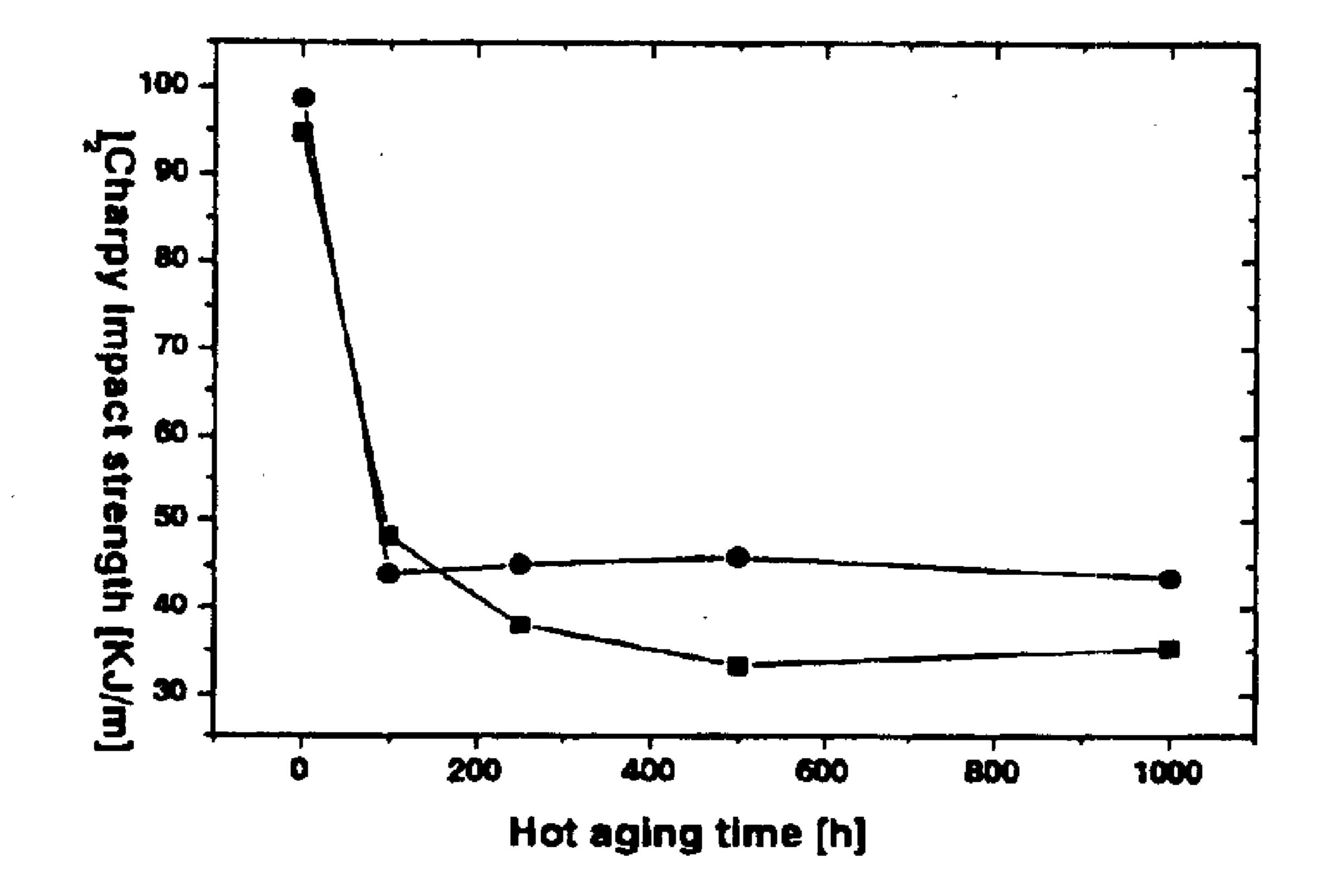
It is clear from FIG. 2 that the polymer prepared according to comparative example 1 exhibits a larger change in the Charpy impact strength than that obtained according to inventive example 1.
