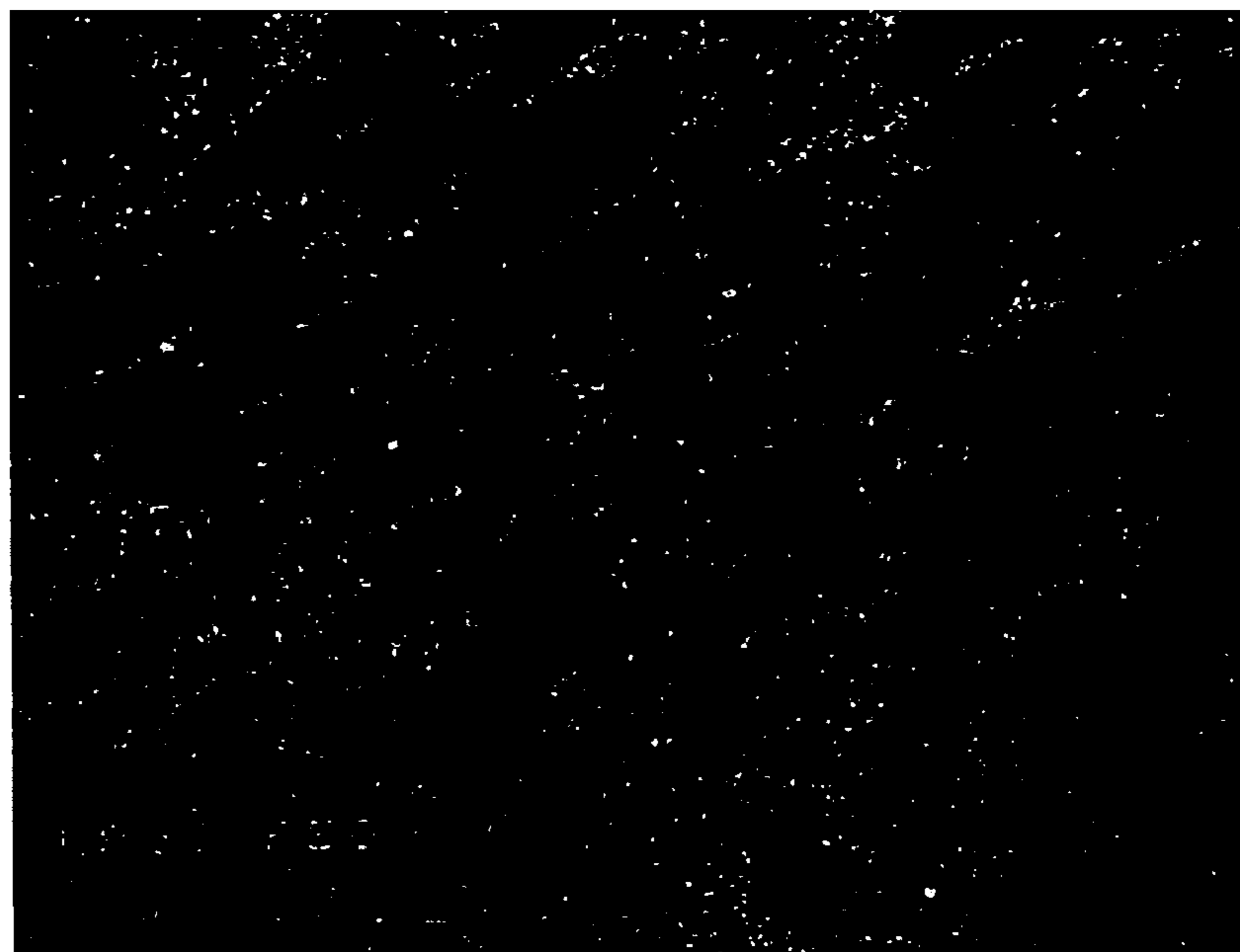
KPO6 PVOH/PEO 70/30 surface, osmicated, compo image, 230x
