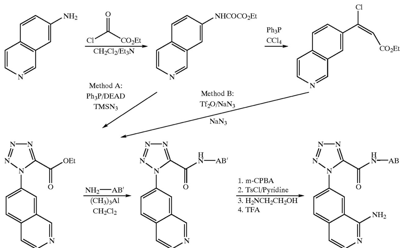
The tetrazole compounds of this invention where Z is —CO— can also be prepared via iminoyl chloride (*Chem. Ber.* 1961, 94, 1116 and *J. Org. Chem.* 1976, 41, 1073) using an appropriately substituted acyl chloride as starting material. The ketone-linker can be reduced to compounds where Z is alkyl.
