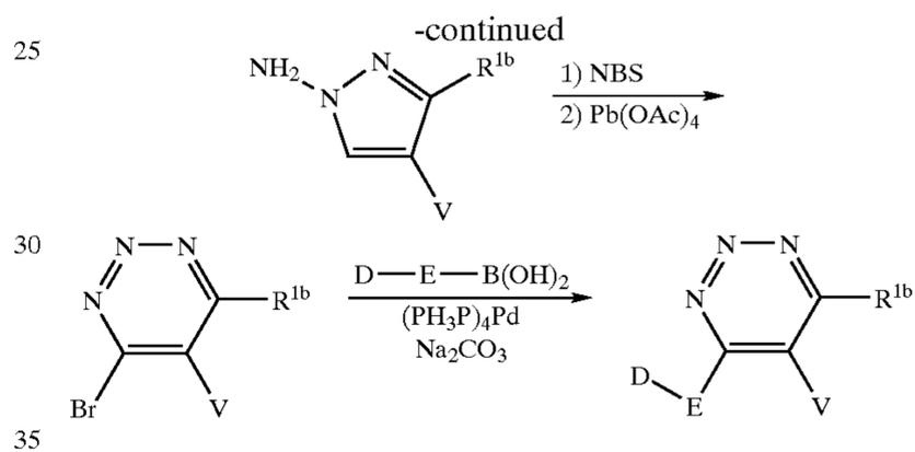
In Scheme 53, an alkene is allylicly brominated and the bromide is displaced to give a regioisomer of the azide in Scheme 52. Following the same reaction sequence as shown above, cyclization provides the 1-aminopyrazole. Bromination followed by lead tetraacetate mediated rearrangement give the 1,2,3-triazine. Palladium-catalyzed coupling provides the other desired triazine.
