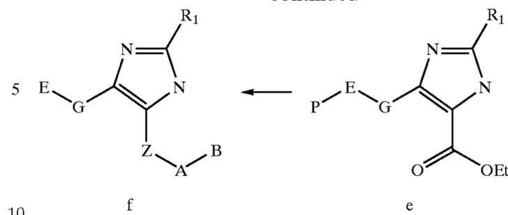
The general procedure to make C-linked imidazole ring **M** is described in Scheme 19. Aldehyde **D-E-CHO** from Scheme 1 can be converted into cyano compound by treatment with hydroxyamine and then dehydration with  $\text{POCl}_3$ . The amidine can be obtained from cyano compound by Pinner reaction, which can be cyclized with  $\alpha$ -halo ester, ketone or aldehyde to form imidazole ring **M**.
