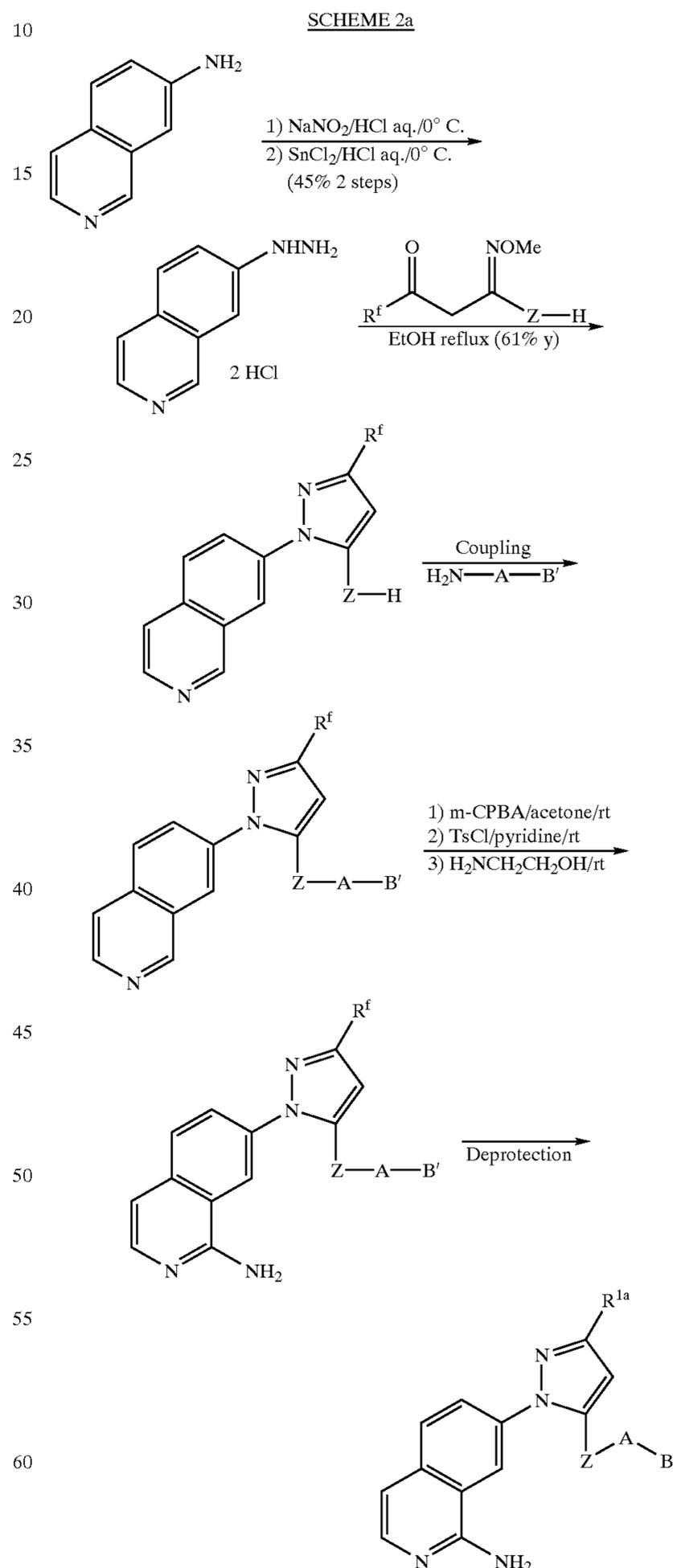
In Scheme 2b is illustrated the preparation of 5-amino substituted 1,6-naphthyridine compounds. Compounds of
