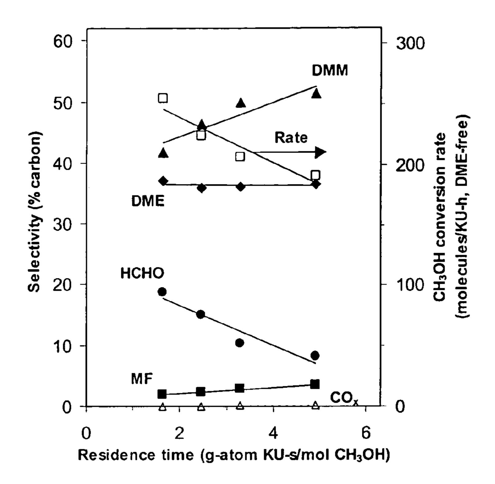
Figure 8. CH<sub>3</sub>OH conversion rates (on a DME-free basis) and selectivities as a function of reaction temperature on H<sub>5</sub>PV<sub>2</sub>Mo<sub>10</sub>O<sub>40</sub>/ZrO<sub>2</sub> (0.31 KU/nm<sup>2</sup>, 4 kPa CH<sub>3</sub>OH, 9 kPa O<sub>2</sub>, 1 kPa N<sub>2</sub>, CH<sub>3</sub>OH conversion: 14.5-51.2%).
