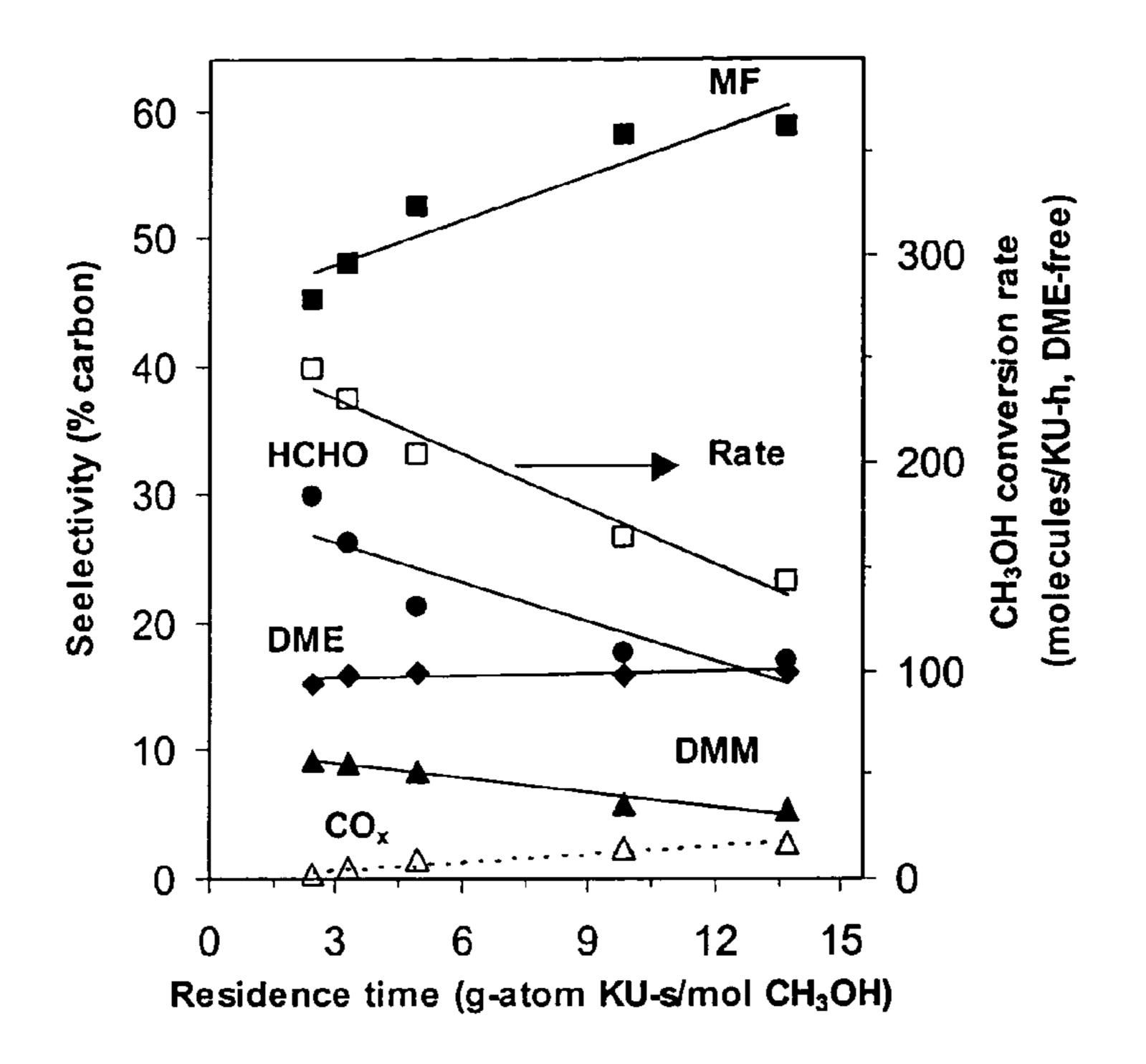
Figure 7. CH<sub>3</sub>OH conversion rates (on a DME-free basis) and selectivities as a function of residence time at 493 K on H<sub>5</sub>PV<sub>2</sub>Mo<sub>10</sub>O<sub>40</sub>/SiO<sub>2</sub> (0.28 KU/nm<sup>2</sup>, 4 kPa CH<sub>3</sub>OH, 9 kPa O<sub>2</sub>, 1 kPa N<sub>2</sub>, CH<sub>3</sub>OH conversion: 21.3-47.6%).
