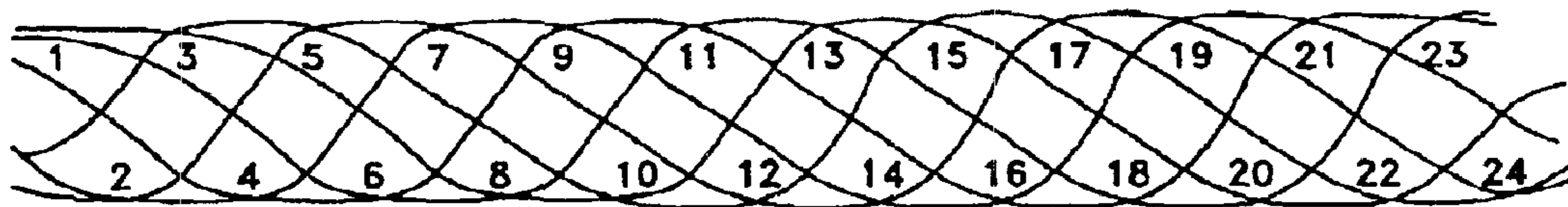
SELF INTERLOCKING TYPE 19 WEAVE
