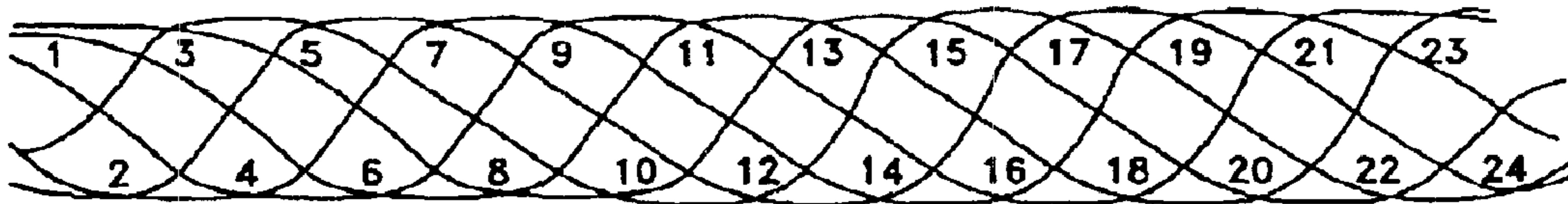
SELF INTERLOCKING TYPE 19 WEAVE
