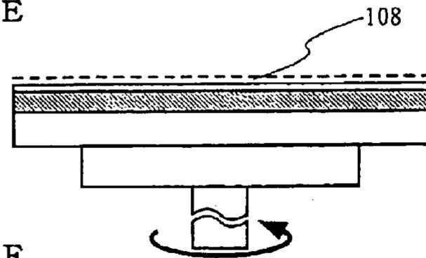
FORMATION OF NICKEL-CONTAINING LAYER BY SPIN DRYING ACCELERATION TO 1200 RPM AT LOW ACCELERATION OF 30 RPM/SEC SPIN DRYING FOR 20 SEC AT 1200 RPM
