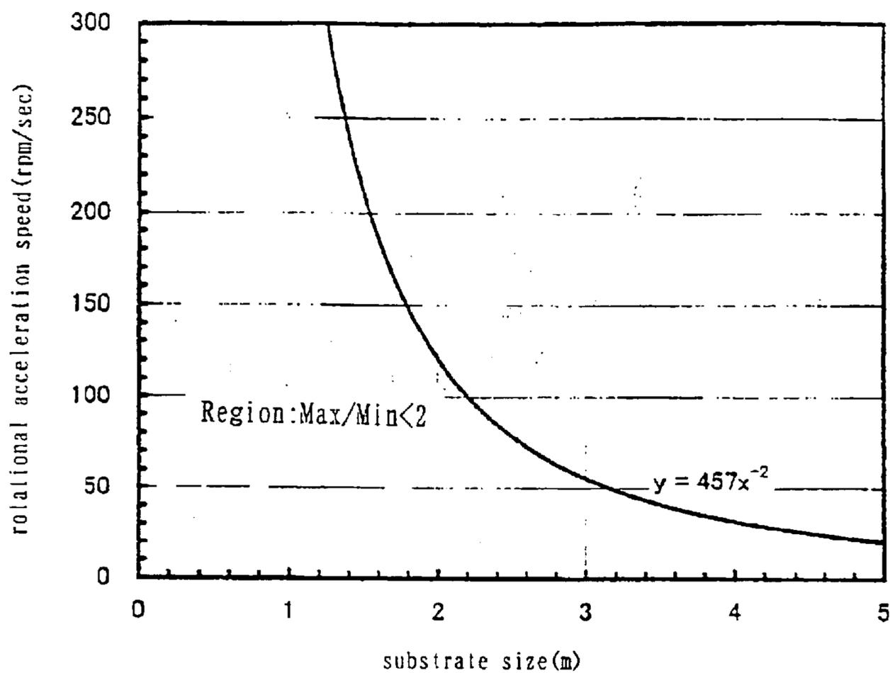
the relationship between substrate size and rotational acceleration speed.
