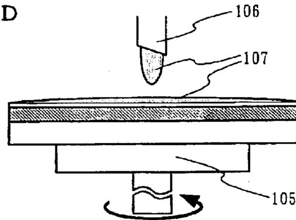
ADDITION OF AQUEOUS NI ELEMENT SOLUTION BY SPIN ADDITION METHOD SPIN ADDITION IN LOW VELOCITY SPIN STATE OF 100 RPM
