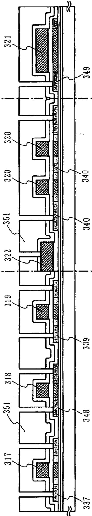
FIG. 11B FORMATION OF METAL WIRINGS /FORMATION OF TRANSPARENT CONDUCTIVE FILM
