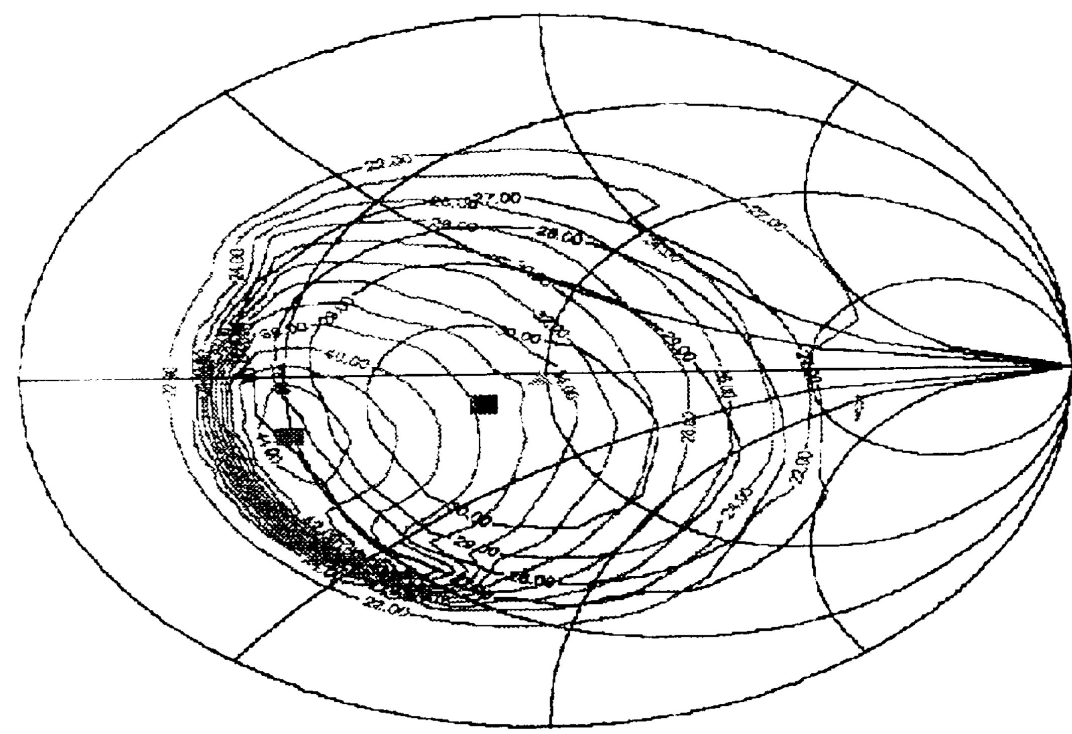
S/N 103 23124u CDMA Fo=836Mhz Pout=28.0dBm Vref=3.1v Vcc=3.5v
