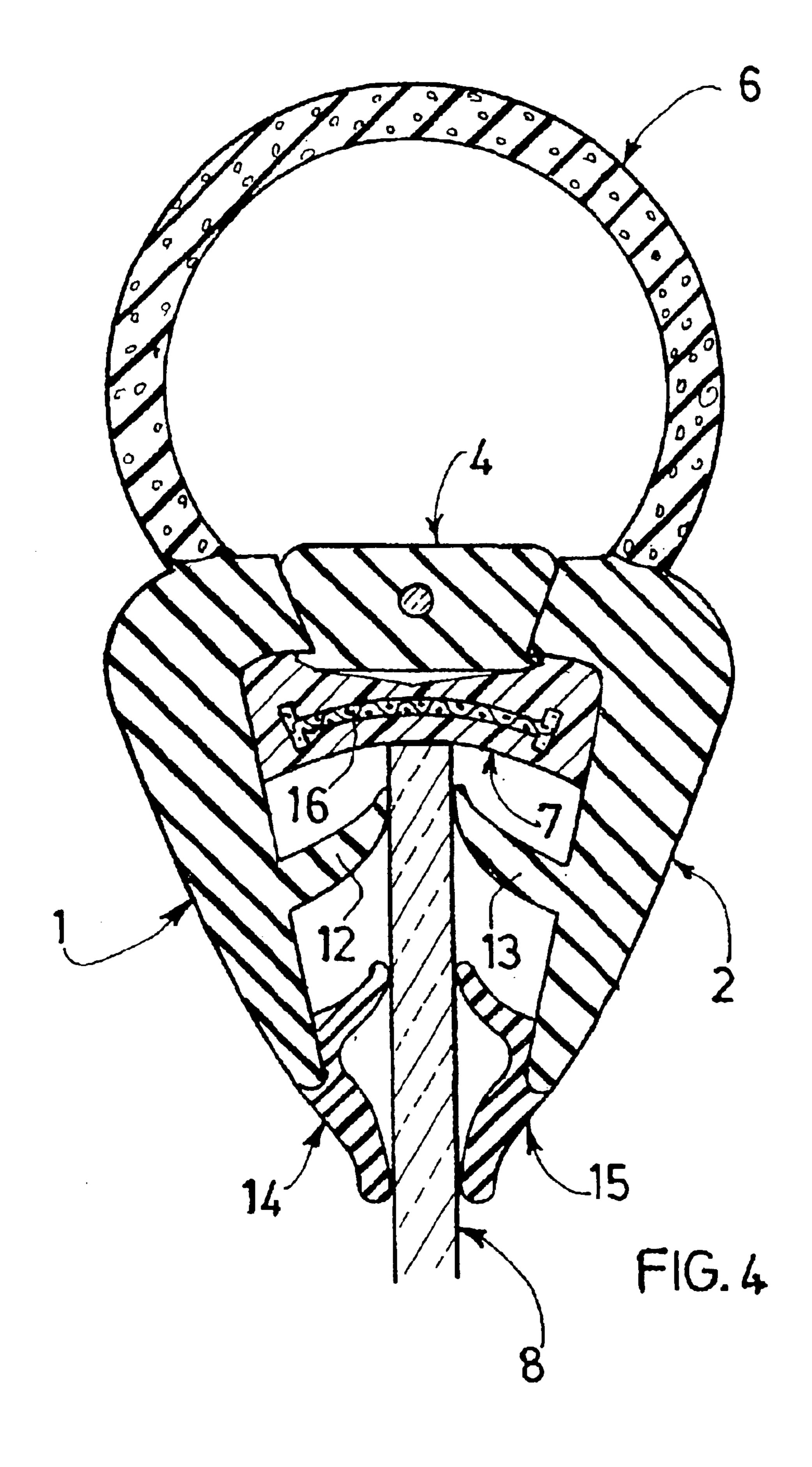
EXTRUDED SEALING SECTION DESIGNED TO BE MOUNTED ON A PROJECTED PART OF A STRUCTURE, PRE-FORM OF SAID SECTION AND PROCEDURE FOR MOUNTING SAID PRE-FORM ONTO THE **PROJECTING PART**
