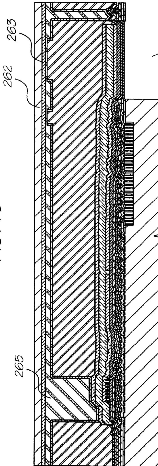
Mount on wafer blank, back-etch inlets
