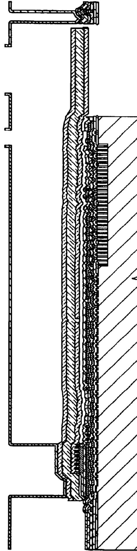
*Detach from wafer blank, etch sacrificial material*
