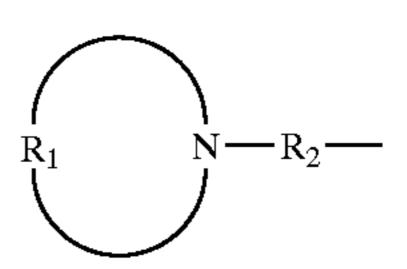
where R<sub>1</sub> is a selected from the group consisting of a divalent alkylene group, an oxy-alkylene group, an amino alkylene group, and a substituted alkylene group, each group having from about 6 to about 20 carbon atoms, R<sub>2</sub> is covalently bonded to the elastomer and is selected from the group consisting of a linear-alkylene group, a branched-alkylene group, and a cyclo-alkylene group, each group having from about 2 to about 20 carbon atoms.
