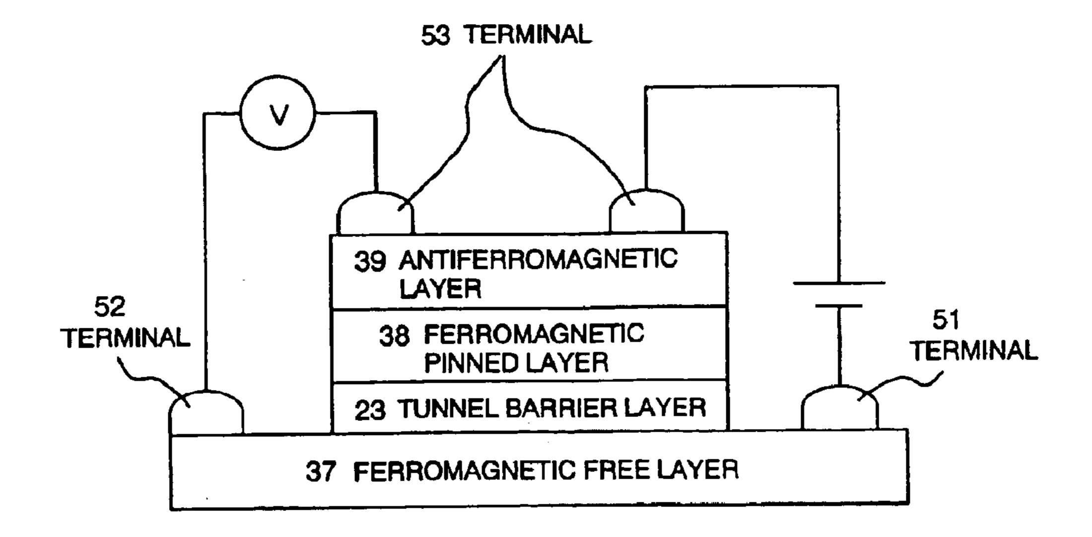
THREE TERMINAL MAGNETIC HEAD HAVING A MAGNETIC SEMICONDUCTOR AND A TUNNEL MAGNETORESISTIVE FILM AND MAGNETIC RECORDING APPARATUS INCLUDING THE HEAD
