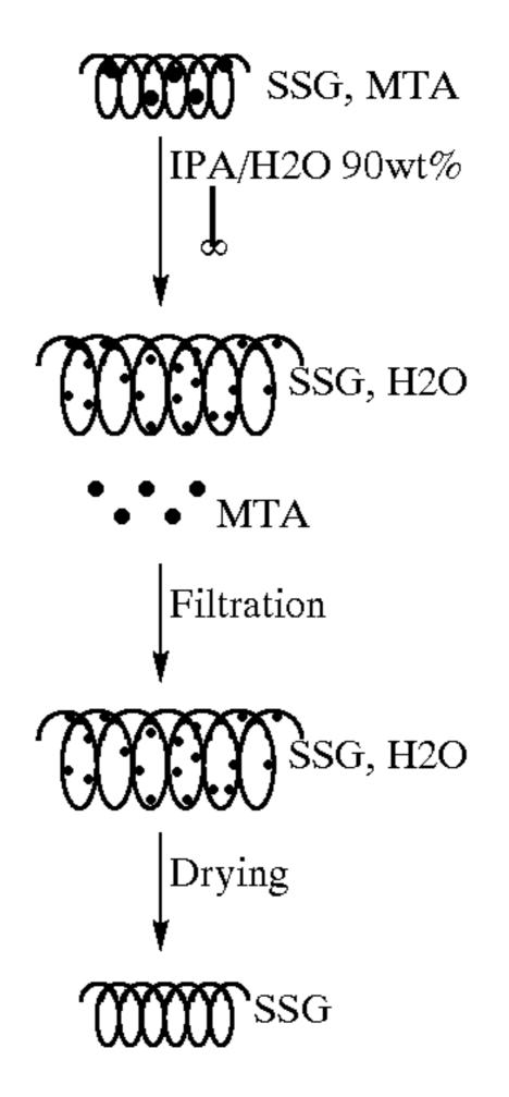
in which SSG represents the modified sodium starch glycolate which contains better water-absorbing property, MTA represents methanol, and IPA represents isopropanol. As shown in this diagram, MTA is initially bonded to the spiral
