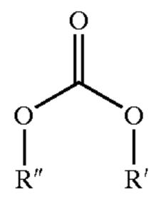
R' and R" independently represent alkyl with up to about 20 carbon atoms, aryl, alkaryl, or aralkyl, R' and R" together with the two oxygen atoms and the carbon atom can form a heterocyclic ring.
