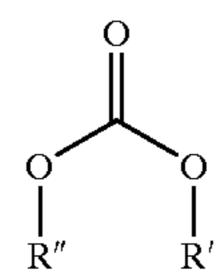
R' and R" independently represent alkyl, aryl, alkaryl, or aralkyl group containing up to about 20 carbon atoms where optionally, R' and R" together with the two oxygen atoms and the carbon atom in the carbonate group can form a heterocyclic ring, and
