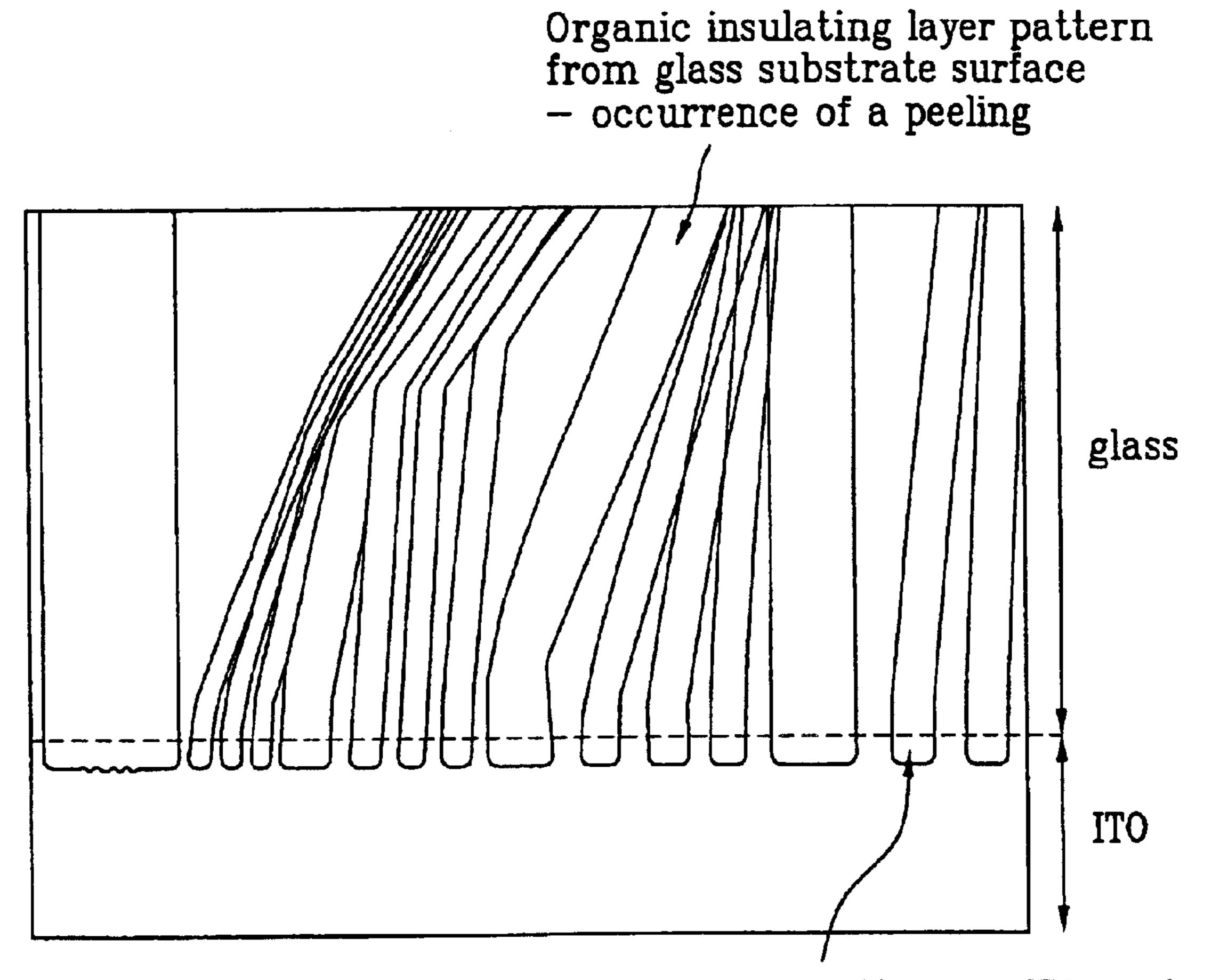
Organic insulating layer pattern on ITO surface — no occurrence of a peeling
