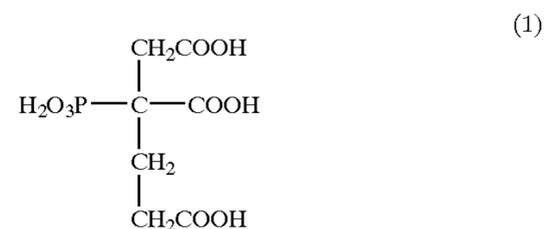
The inkjet recording head is treated with the organic phosphonic compound represented by formula (1) so that the surface of a heater device of the inkjet recording head is treated with the organic phosphonic compound represented by formula (1).
