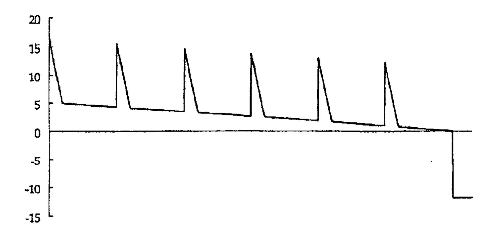
Conditions - Triangular wave 5ASD with 11.25ASD multi-peak and 12ASD reverse current density 80min(with agitation and vibration)
