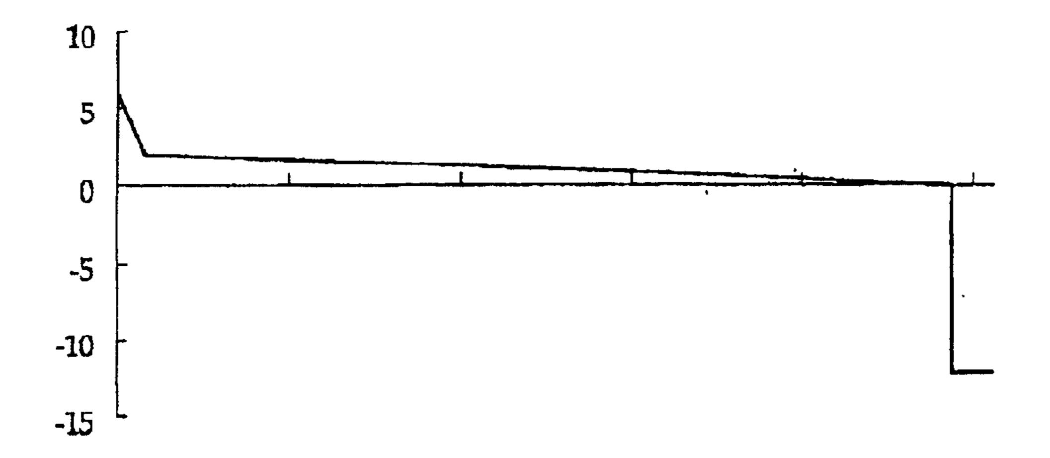
Conditions - Triangular wave 2ASD with 12ASD reverse current density (with agitation)
