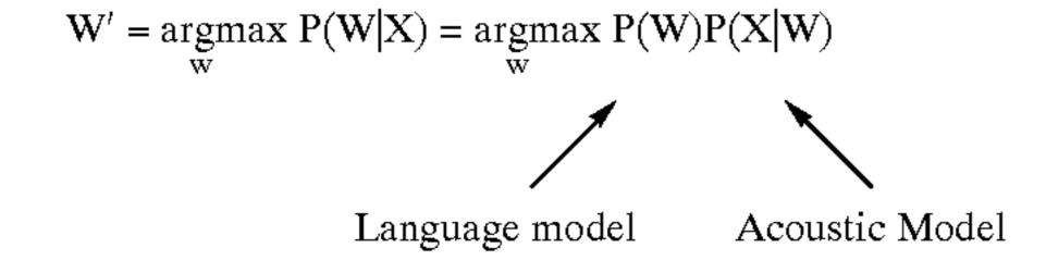
Namely, a probability P(X|W) of said feature (X) when a word sequence W is spoken can be multiplied by a probability of W itself (P(W)). The word sequence W' which makes the multiplication product the largest (argmax) can be selected as a recognition result.
