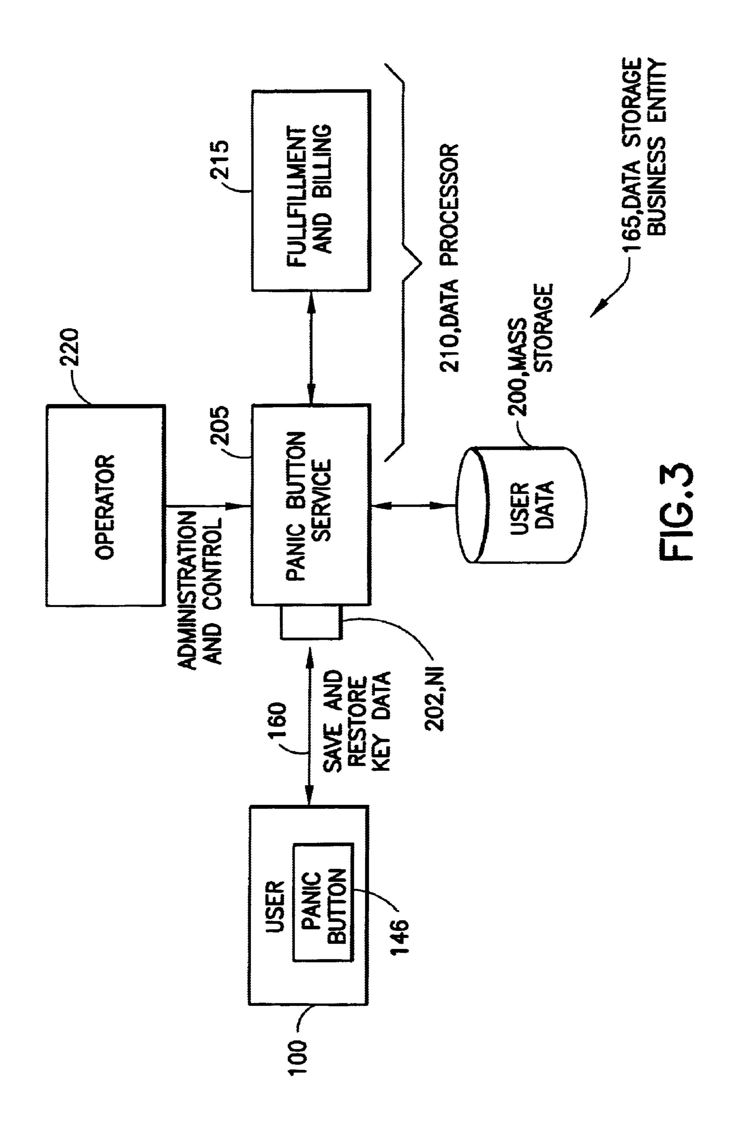
METHOD AND APPARATUS FOR PERFORMING EMERGENCY SHUTDOWN OF A MALFUNCTIONING COMPUTER SYSTEM SAVING ALL OPEN FILES, DATA, AND WORK IN PROGRESS TO A REMOTE DATA STORAGE BUSINESS ENTITY
