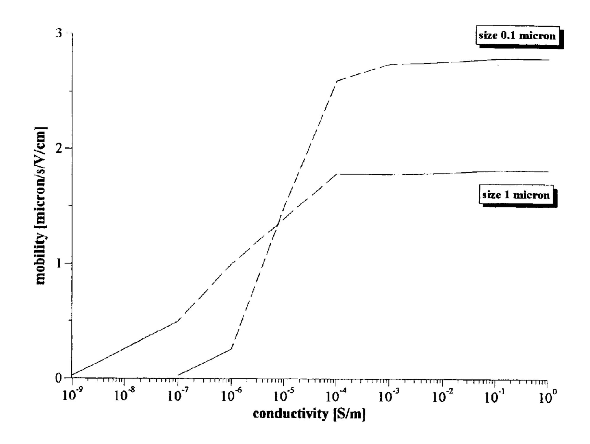
Figure 3. Electrophoretic dynamic mobility at 3 MHz of the barium titanate particles in water at 10% weight, temperature 22  $C^0$ ,  $\zeta$ -potential is 25 mV. Particles density is 5 g/cm<sup>3</sup>, dielectric permittivity 1000. Density of water is 0.997 g/cm<sup>3</sup>, dielectric permittivity is 79.9, dynamic viscosity is 0.94 cp
