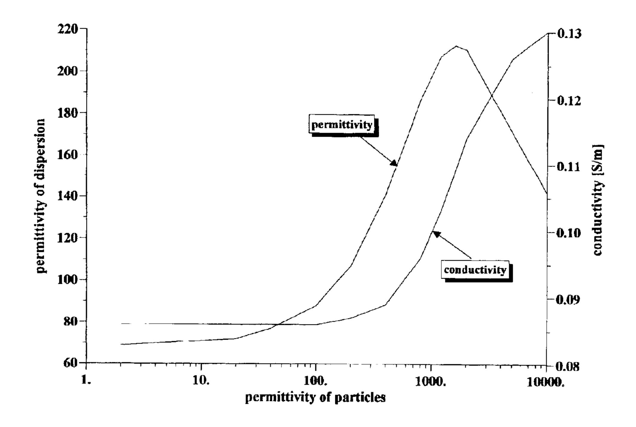
Figure 5. Verification of Maxwell-Wagner theory with aluminum hydroxide particles in water. Particle diameter is 1 micron. Two ways equilibrium dilution with supernate: from high concentration (76%wt) to lower by adding supernate to the initially concentrated dispersion, and from low concentration to higher by adding concentrated dispersion to the supernate.. Conductivity is measured at 3 MHz.
