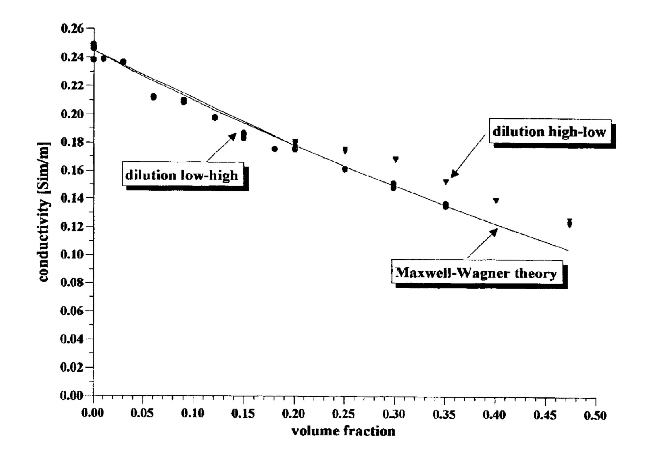
Figure 6. Colloid Vibration Current measured for iron oxide particle 15 nanometer in size in toluene-bitumen mixture with surfactant presence for various weight fractions of particles.
