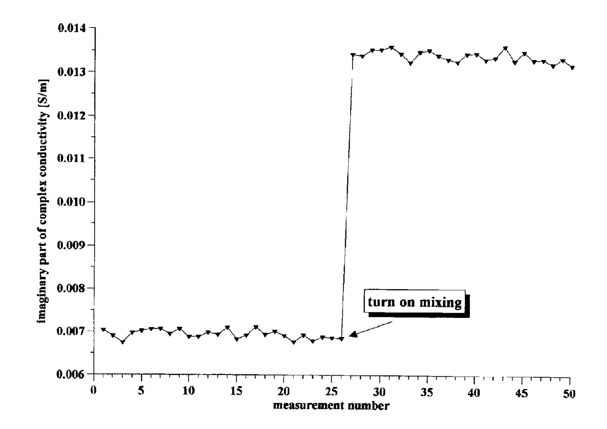
Figure 9. Titration of 20%wt barium titanate slurry. Electroacoustic and conductivity measurements are made with DT-1200 by Dispersion Technology Inc. Dielectric permittivity of particles for calculating  $\zeta$ -potential is assumed as 850.
