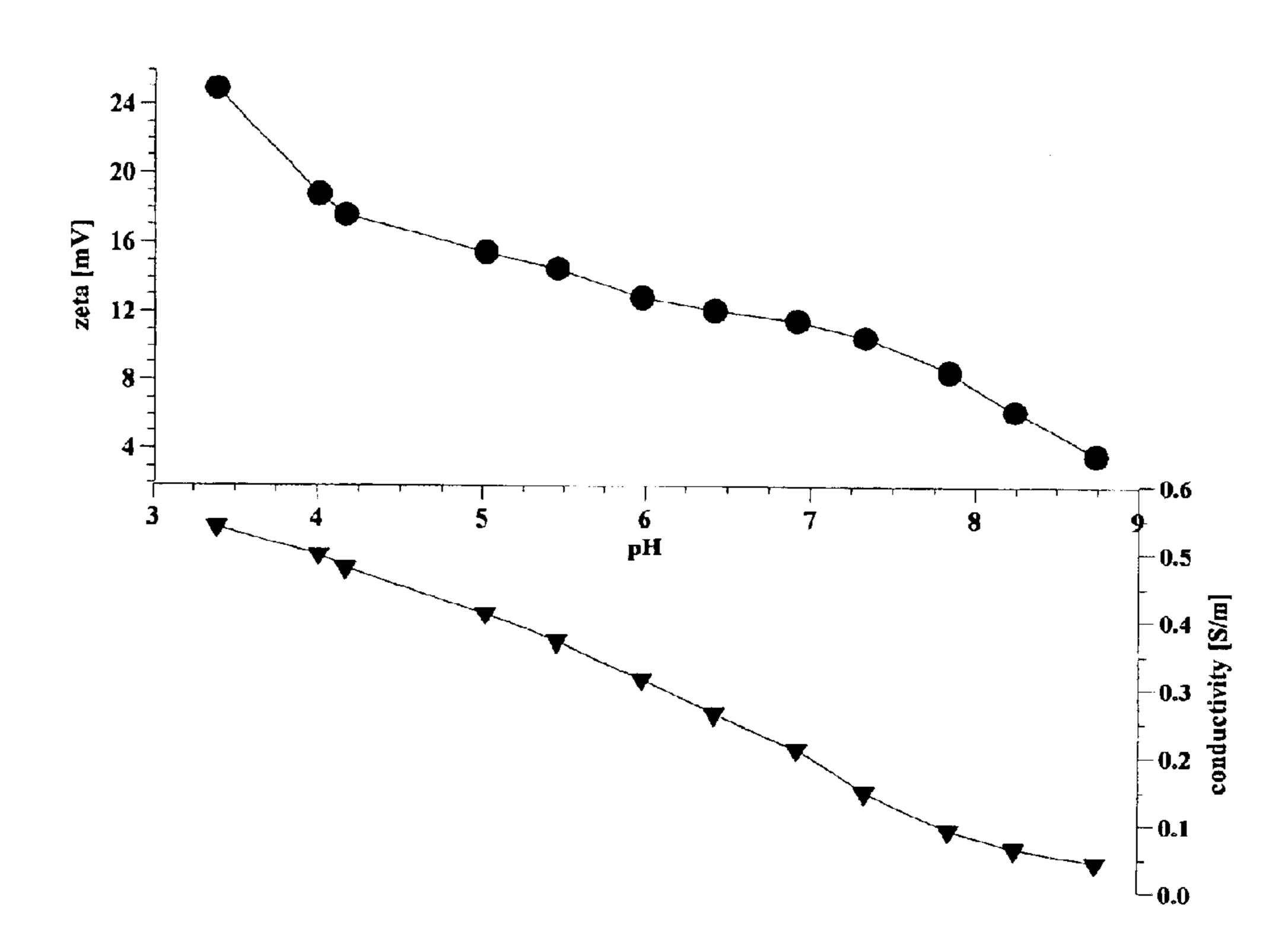
Figure 10. Titration of 20%wt barium titanate slurry. Measurement of Colloid Vibration Current phase is made with DT-1200 by Dispersion Technology Inc. Dielectric permittivity of particles for calculating theoretical phase is assumed as 850 and 3.
