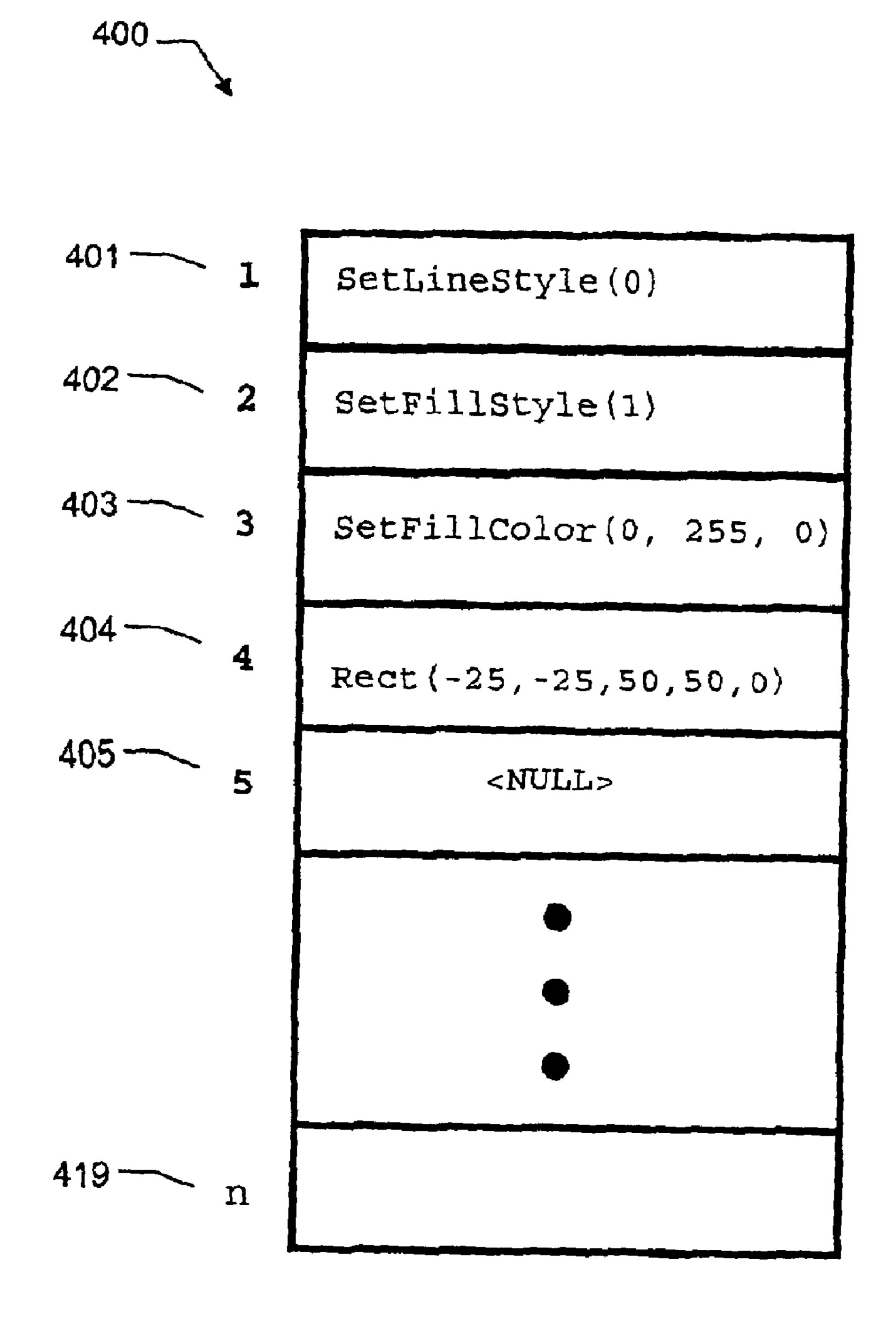
FIG. 4 - Display List Data Structure
