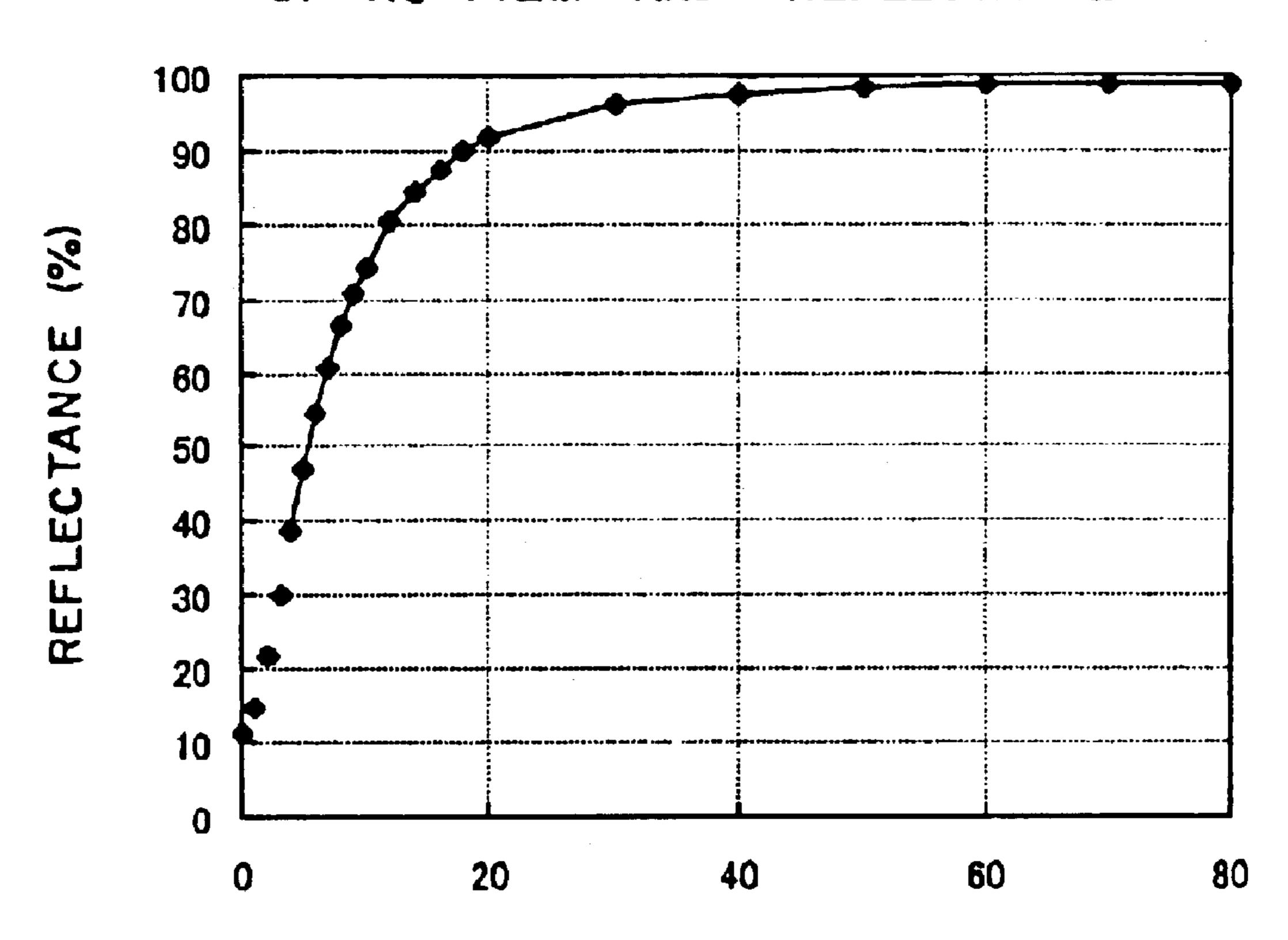
THICKNESS OF Au FILM (nm)
