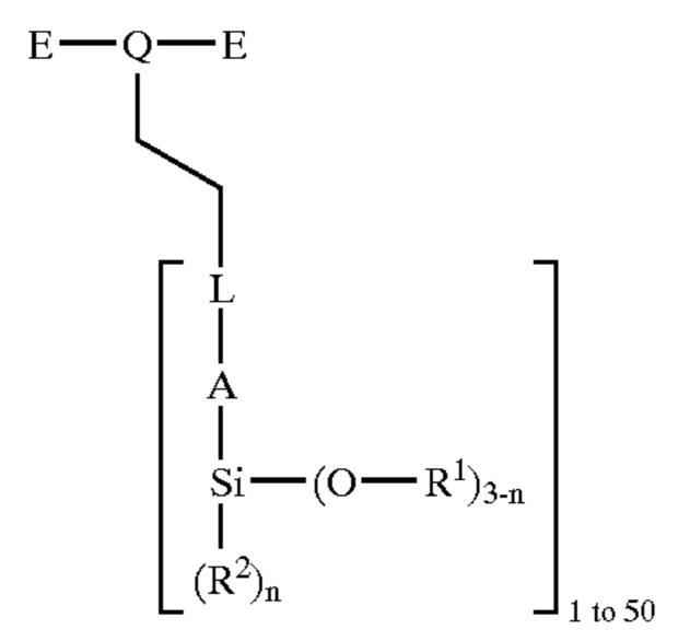
in which E is an electron donor or electron acceptor functionality; Q is an oligomeric or polymeric group containing at least one carbon to carbon double bond, A is a hydrocarbyl group; and L is a linking group.
