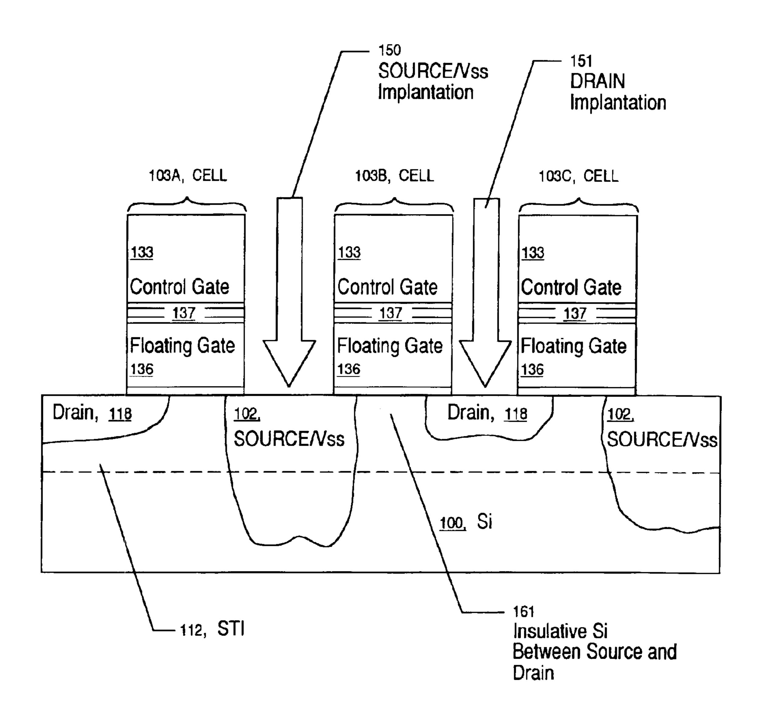
FIGURE 1C CONVENTIONAL ART (SECTION B-B)
