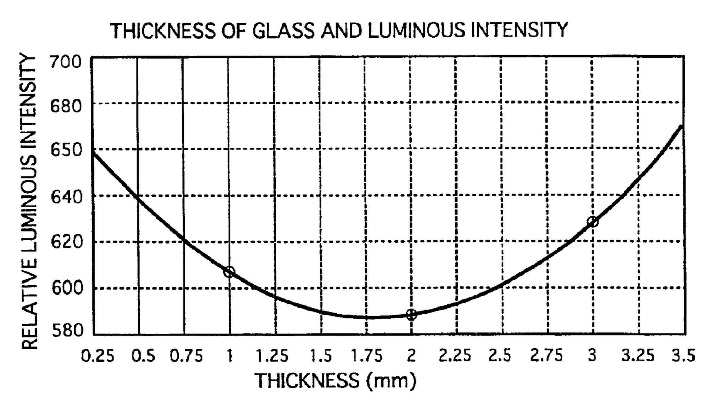
O EMISSION LIGHT AMOUNT— EMISSION LIGHT CURVE BASED ON MEASURED LIGHT AMOUNT
