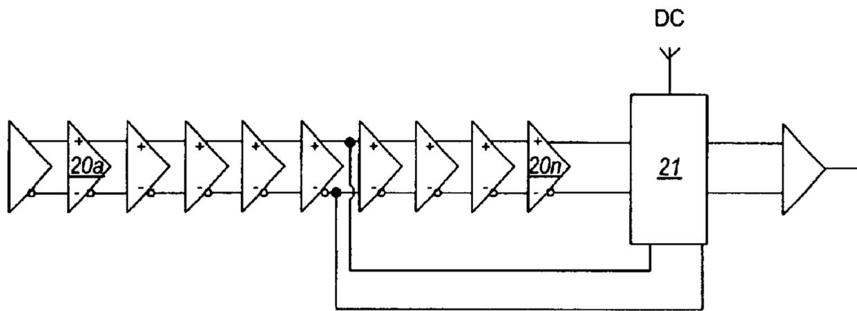
DELAY LINE WITH DELAY CELL SWITCHING CIRCUIT
