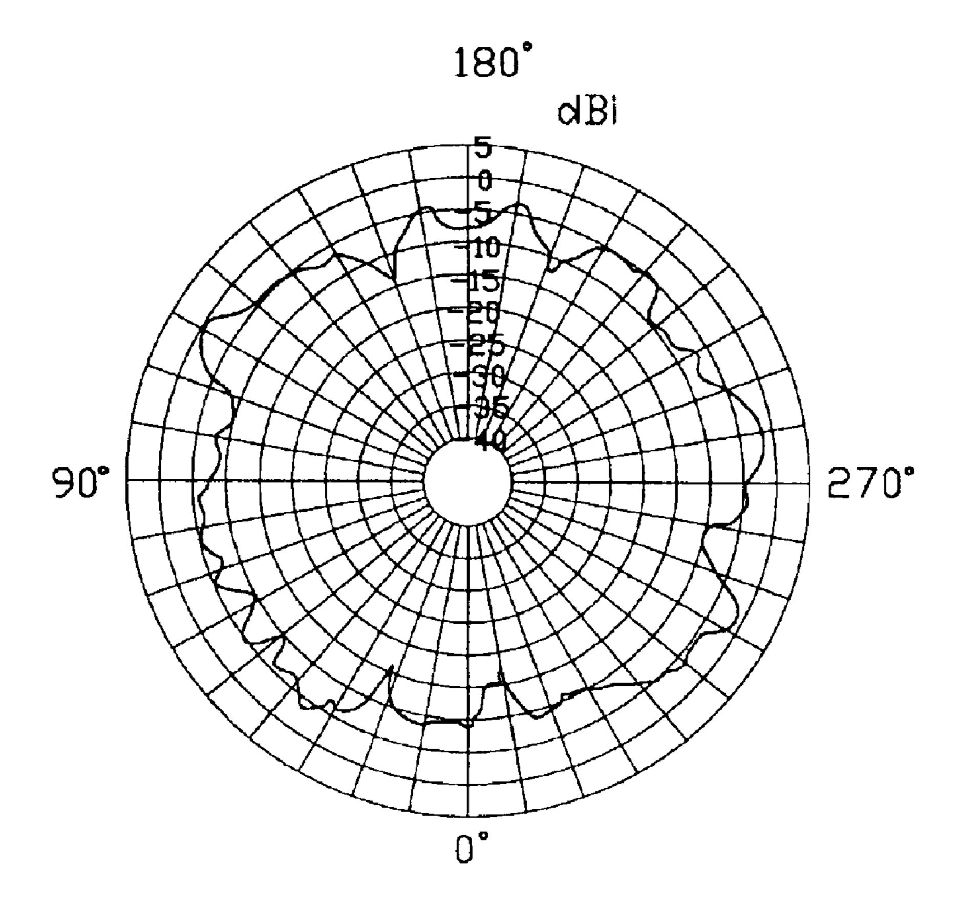
Scale 5 dBI/div Operating Frequency: 5.725 GHz Vertically Polarized
