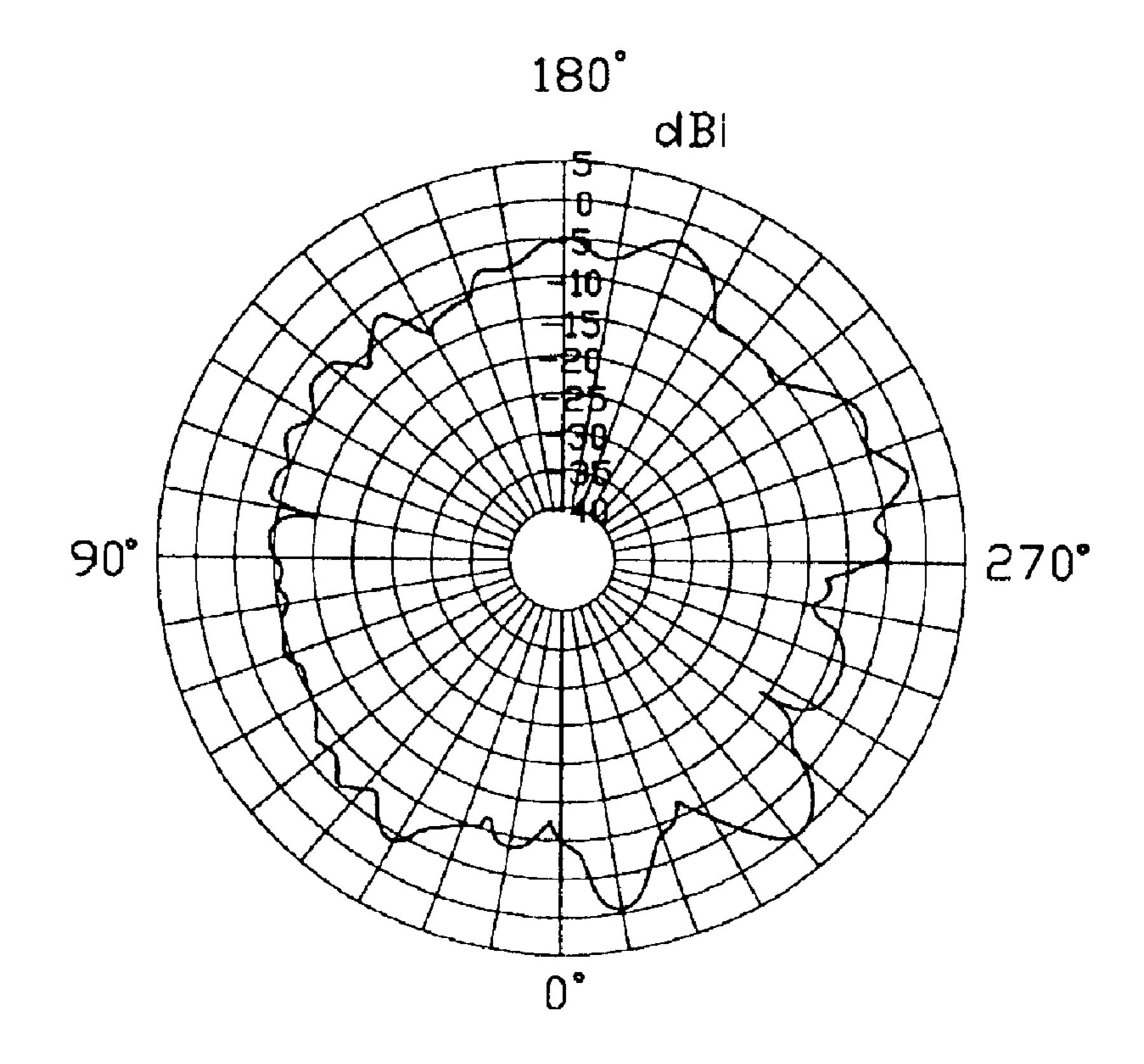
Scale: 5 dBi/dlv Operating Frequency: 5.725 GHz Horlzontally Polarized
