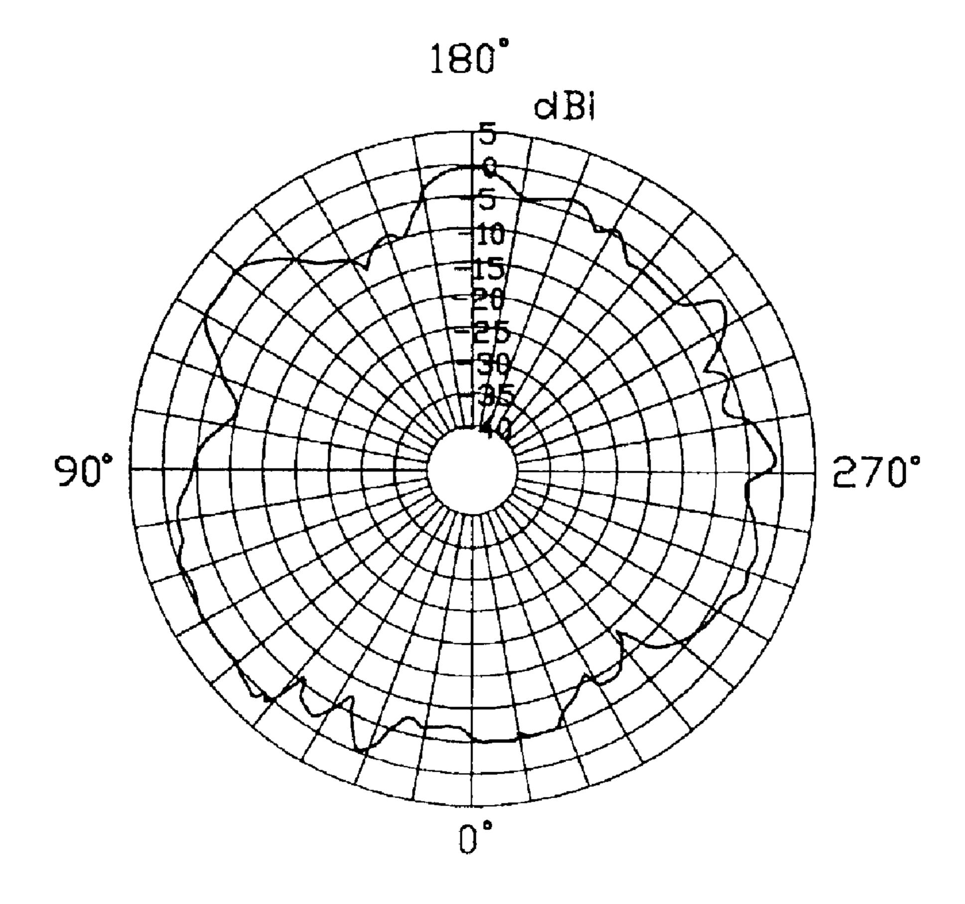
Scale: 5 dBI/dIv Operating Frequency: 5.35 GHz Vertically Polarized
