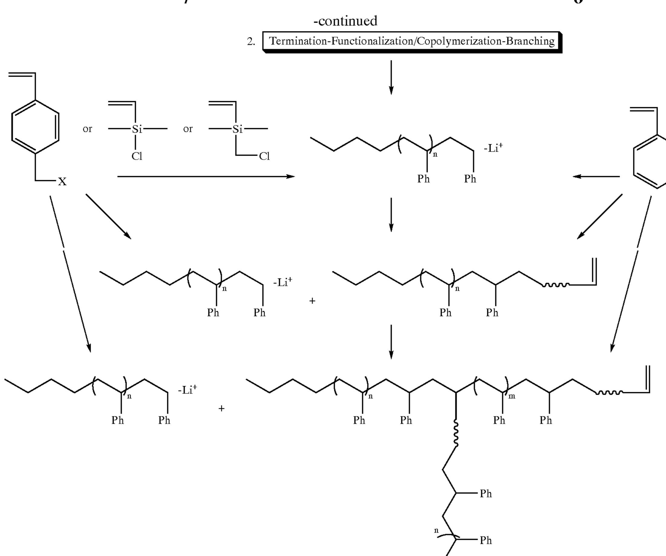
Polystyrenes with molecular weights in the range 3,000–60,000, polydispersity <2.5 with 5 to 40 branches, each containing 3 to 30 monomer units were prepared, primarily controlled by the initiator/monomer/chain terminating agent ratio, relative addition rates, the reactivity ratios of the macromonomer and (co)monomers.
