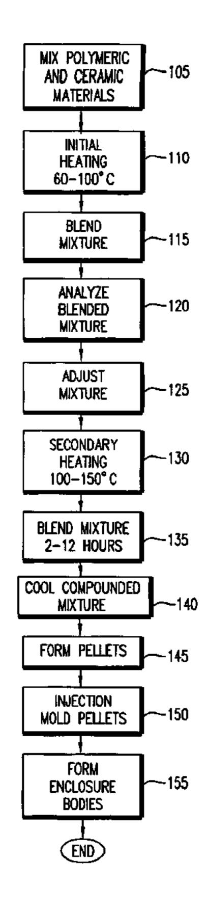
MIX POLYMERIC AND CERAMIC MATERIALS INITIAL HEATING 60-100°C BLEND MIXTURE **ANALYZE** BLENDED MIXTURE **ADJUST** -125**MIXTURE** SECONDARY HEATING 100-150°C BLEND MIXTURE 2-12 HOURS COOL COMPOUNDED MIXTURE <del>--140</del> FORM PELLETS INJECTION MOLD PELLETS FORM **ENCLOSURE BODIES**
