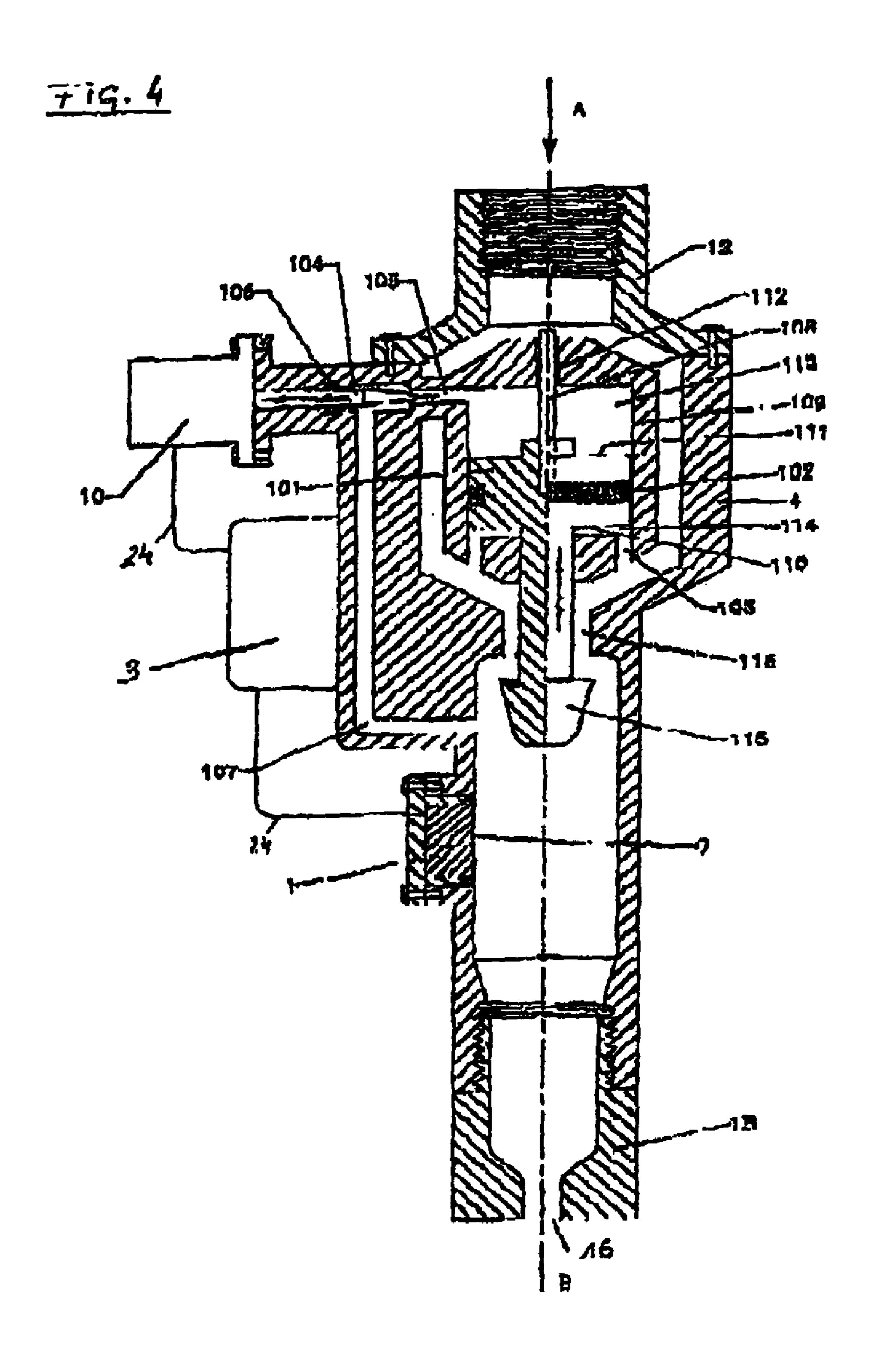
The invention concerns a valve for a liquid or gaseous medium comprising a movable valve body, by way of which the internal through-flow cross-section is adjustable.
