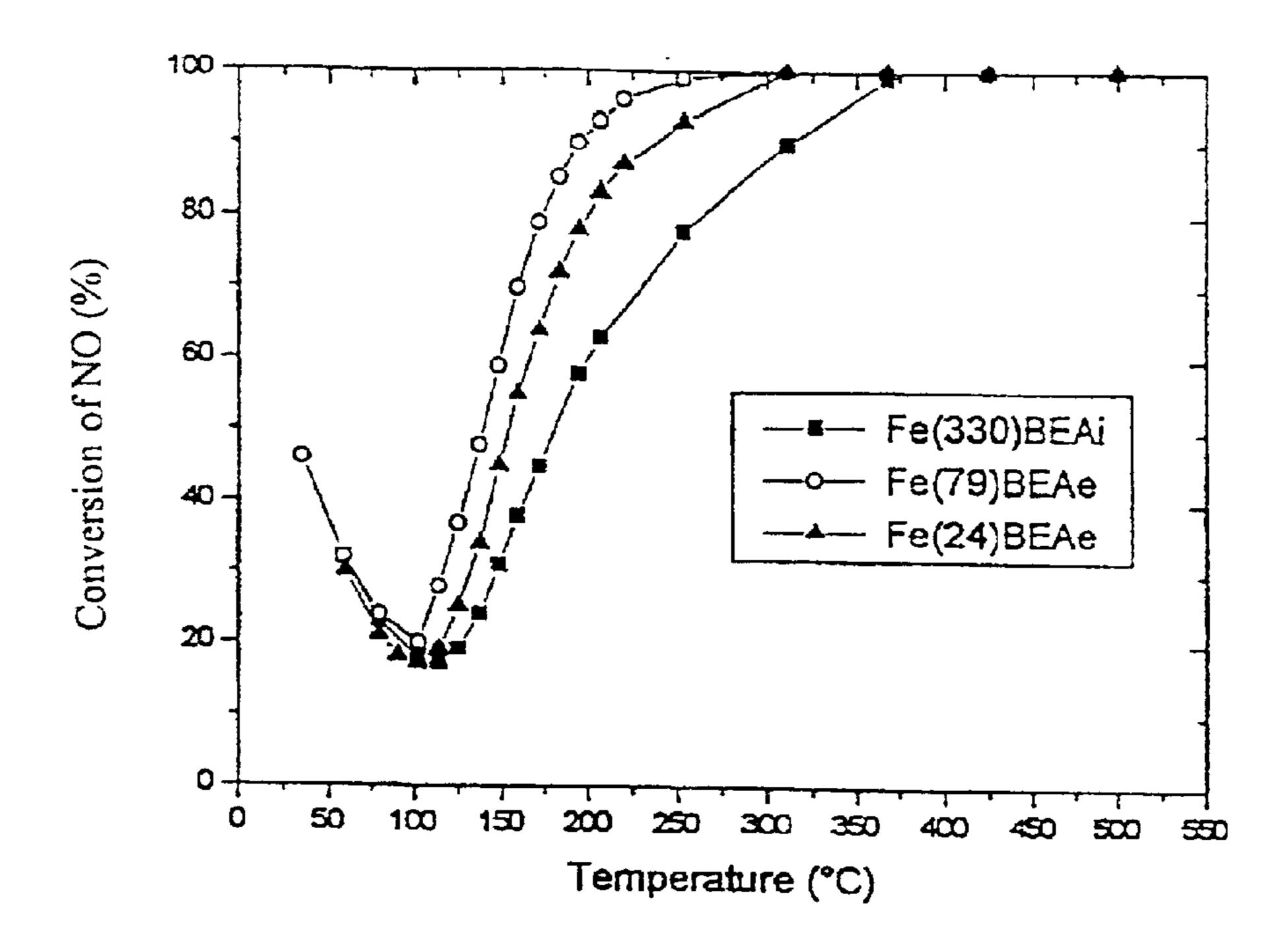
Fig. 3c: Simultaneous elimination of NO and N<sub>2</sub>O on FeBEA VVH =  $10000 \text{ h}^{-1}$ , 3% 0<sub>2</sub>, 13500 pm H<sub>2</sub>O, 1500 ppm NO, 1000 ppm N<sub>2</sub>O, 2500 ppm NH<sub>3</sub>, 1 hour stage every 10°C
