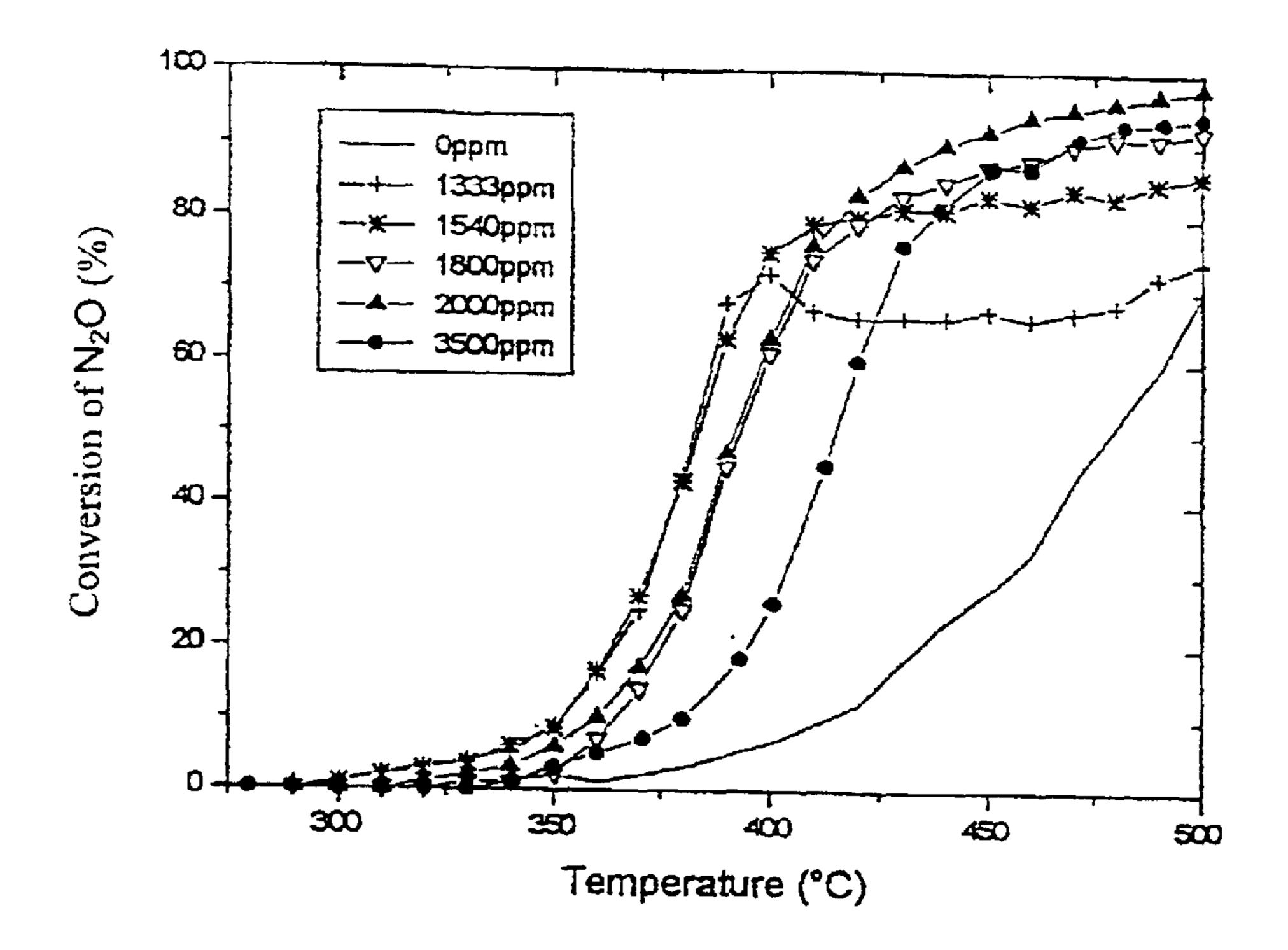
Fig. 2b1: Influence of the NH<sub>3</sub> content on the SCR of  $N_2O + NO$  Effect on the NO conversion of  $N_2O$ ; VVH =35000 h<sup>-1</sup>; 3%  $O_2$ , 2000 ppm  $N_2O$ , 500 ppm NO, x ppm
