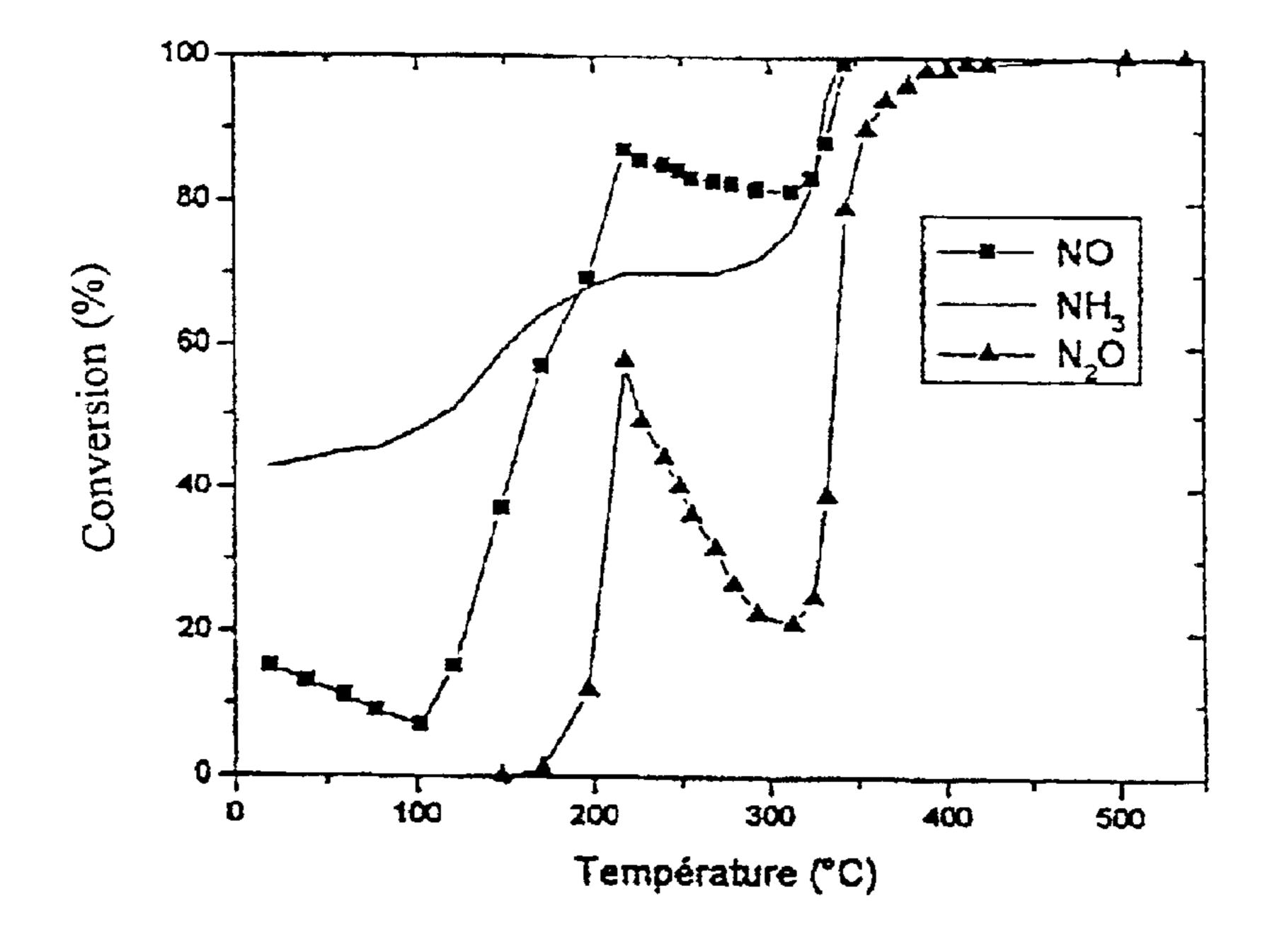
Fig. 4: Influence of the preparation method on SCR of N<sub>2</sub>O + NO VVH = 35000 h<sup>-1</sup>, 3% 0<sub>2</sub>, 2000 pm N<sub>2</sub>O, 500 ppm NO, 1333 ppm NH<sub>3</sub>; stage 1h/10°C Catalyst: Fe(49) BEA<sub>e</sub>; prepared by exchange and Fe(51) BEA; prepared by impregnation
