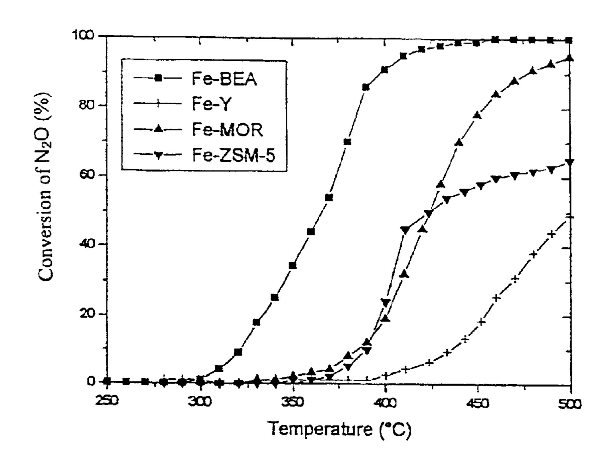
Fig. 2a: Influence of the presence of NH<sub>3</sub> on the catalytic elimination of N<sub>2</sub>O in the presence of 3% O<sub>2</sub>, VVH = 35000 h<sup>-1</sup>, 3% O<sub>2</sub>, 2000 ppm N<sub>2</sub>O, He.
