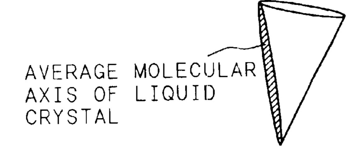
WHEN VOLTAGE OF SECOND POLARITY IS APPLIED. FOR EXAMPLE. VOLTAGE V<0
