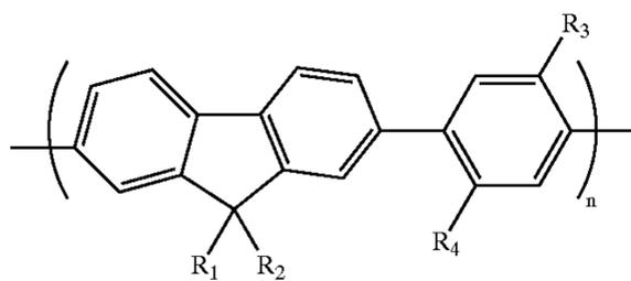
wherein  $R_1$  and  $R_2$  which may be identical or different, are each H, a ( $C_1-C_{22}$ ) linear or branched alkyl, alkoxy or oligo (oxyethylene) group, a ( $C_6-C_{30}$ ) cycloalkyl group, or an unsubstituted or substituted aryl group; wherein  $R_3$  and  $R_4$ , which may be identical or different, are each a linear or branched octoxyl group; and wherein  $n$  is from about 3 to about 5000.
