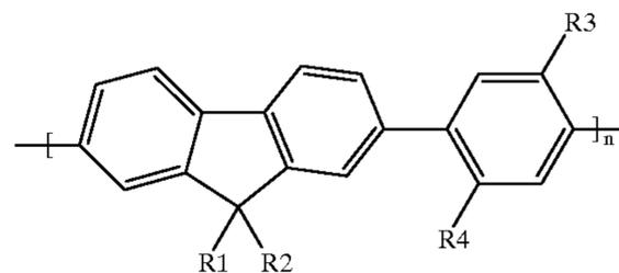
wherein R<sub>1</sub>, R<sub>2</sub>, R<sub>3</sub> and R<sub>4</sub>, which may be identical or different, are each selected from the group consisting of H, a (C<sub>1</sub>–C<sub>22</sub>) linear or branched alkyl, alkoxy or oligo (oxyethylene) group, a (C<sub>6</sub>–C<sub>30</sub>) cycloalkyl group, and an unsubstituted or substituted aryl group, and n is from about 3 to about 5000.
