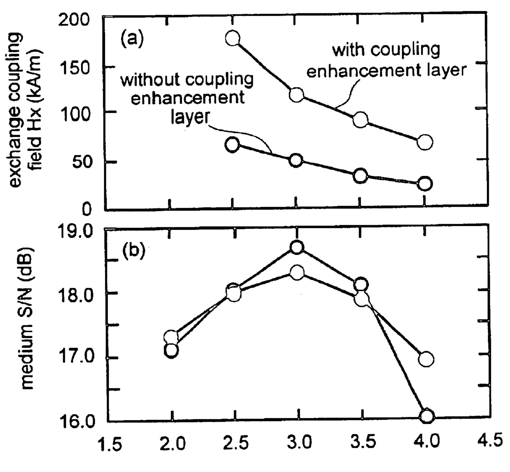
film thickness of lower magnetic layer t2 (nm)
