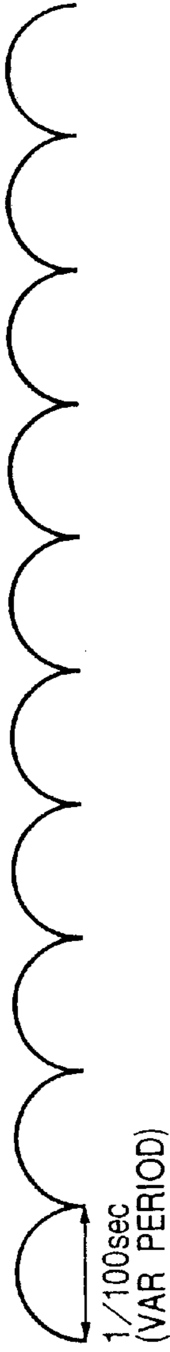
FIG. 3B PRIOR ART LUMINANCE OF FLUORESCENT LAMP
