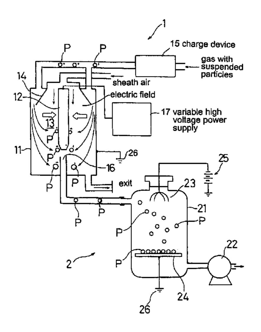
Fig. 1 15 charge device gas with suspended particles Q<sup>+</sup> 14 sheath air electric field 17 variable high voltage power supply 11-′σ́~ /26 25 exit 202020
