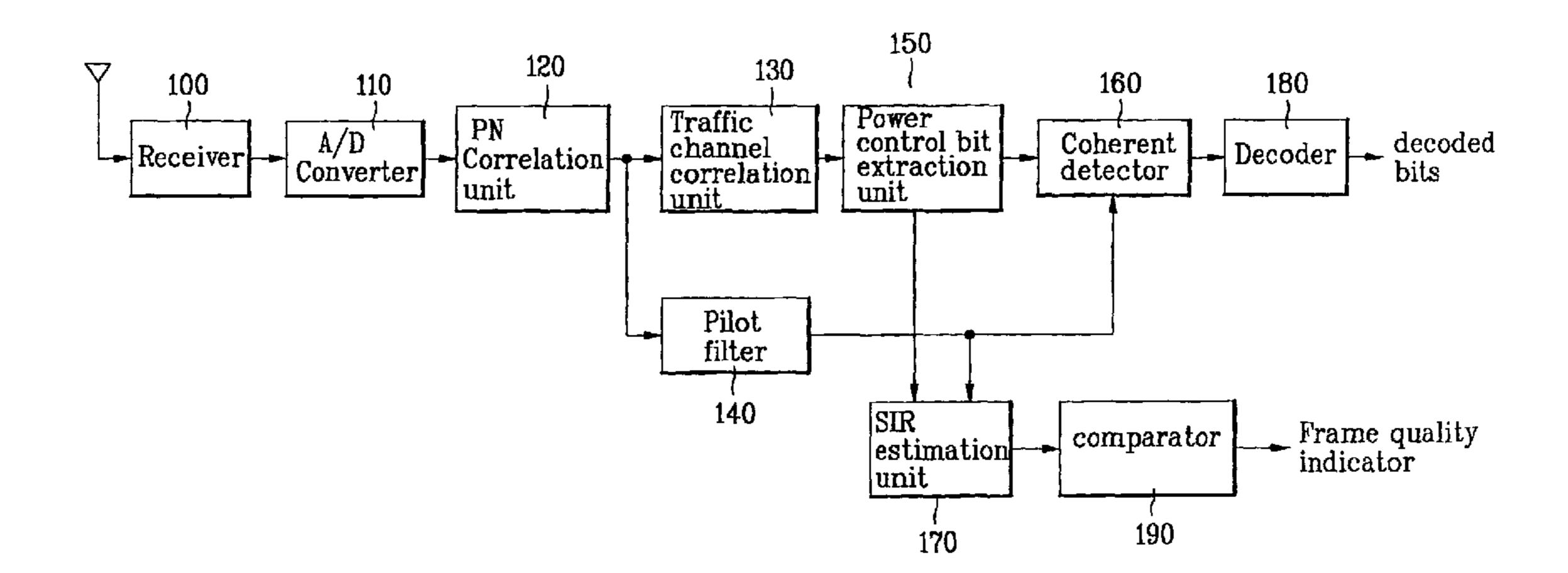
decoded bits ecoder comparator Coherent detector 190 SIR estimation unit Power control bit extraction unit Traffic channel relation 130 Pilot filte unit
