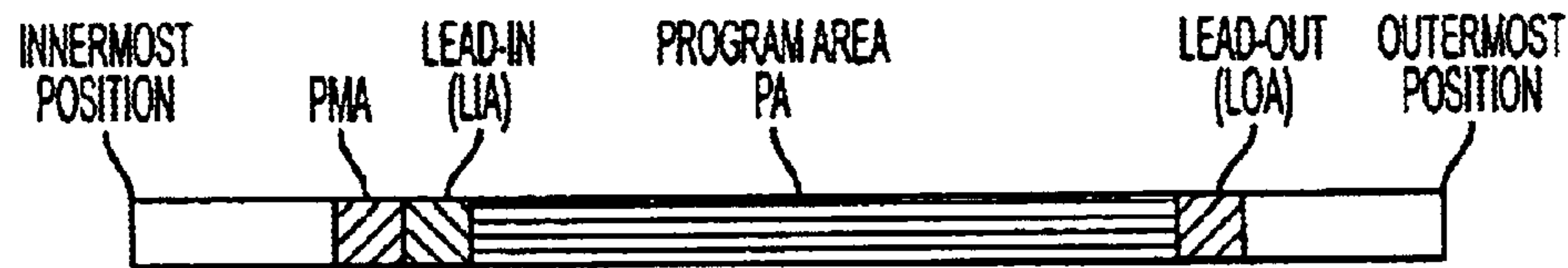
CD-R COMPLETELY RECORDED DISC FIG. 5C
