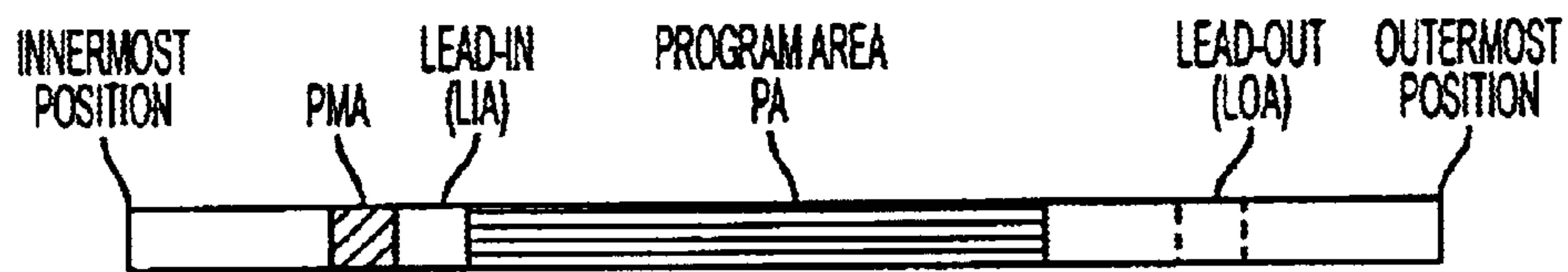
CD-R PARTIALLY RECORDED DISC (PRD) FIG. 5B
